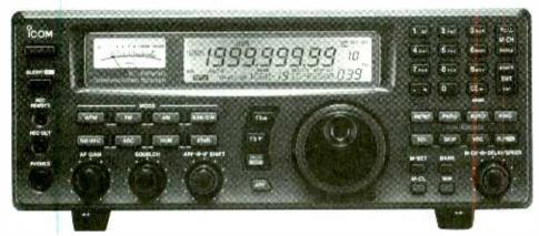
ICOM IC-R8500 and other receivers with SSB product detectors can be used to scan ASCB communications.
