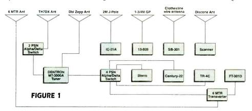
l shows how my antennas are arranged. For HF I use three primary antennas: a HyGain TH7DX 7 element Yagi-Uda type beam antenna for 20/15/10 meters, and an extended double-Zepp for 160/80/ 40/30 meters. A three element 6 meter beam by MFJ sits above the TH7 to give me directional capabilities on the "magic band."
