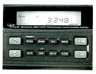
The PRO-2050 is lightweight because there is no chassis and the case is entirely plastic. Power is furnished by an included 12 VDC wall wart. Components are surface mounted on a main printed circuit board and a second board located behind the front panel. We connected a CTCSS display to the discriminator using the solder pad shown here, though this may void the warranty.
