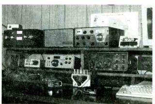
The current line-up at K7SZ, L-R from The top: Denton MT3000A tuner, Drake MS-4 speaker, Drake TR4C HF SSB/CW transceiver. 2nd shelf: amplified speaker, Wilderness Radio Sierra, Ten-Tec Century-22 and Yaesu FT301D HF transceivers. The Ten-Tec 1208 6m is off camera. Note the Alpha Delta four-position RF switch which controls the antennas.
