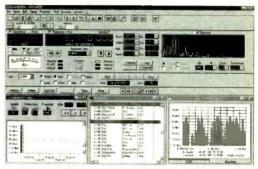
dows based control software for computer-capable scanners and receiver/transceivers from AOR, ICOM, Kenwood, Racal and Yaesu, plus the WiNRADiOcard. Rhode & Schwartz and Watkins Johnson models are supported by the PRO version. The PLUS version of VisualRadio enables use of two other valuable radio accessories: the AOR SDU-5000 spectrum display unit and the Optoelectronics Scout frequency
