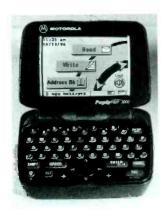
The user can receive messages, respond to those messages, and initiate customized messages. An Intel microprocessor and a software development kit (SDK) allow programmers to use industry-standard development tools to create additional applications.
