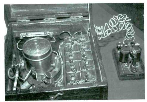
The inside of a Marconi receiver of the type used in his London GPO demonstration, 1896.
