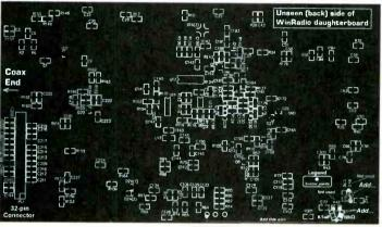
Angle it slightly as shown in Figures 1 and 2. 6. Solder one end of the 12-kohm (size 0805) chip resistor to right-unused pad of R48. Angle it slightly so that its unsoldered end touches the unsoldered end of the 0.1- $\mu F$  capacitor installed in Step 5.
