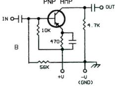
FIGURE 2 — Example of how a positive power supply polarity can be used with NPN or PNP transistors. See text for more information.
