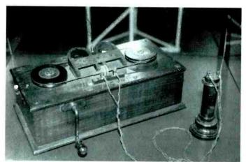
Single earphone magnetic detector. Definitive model produced by Marconi in 1902 at the Laboratory of the Italian Navy.
