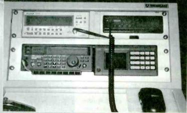
Left: While there are already systems available for broadcasting digital shortwave, you still have to improvise quite a bit when trying to demodulate the signal back into audio: During the digital test in Nauen, two professional EKD 500 receivers - top of the line communications receivers built during the late German Democratic Republic — were used for receiving the signal. It was then fed into computers for the demodulation process before the final result could be broadcast by the speakers.
