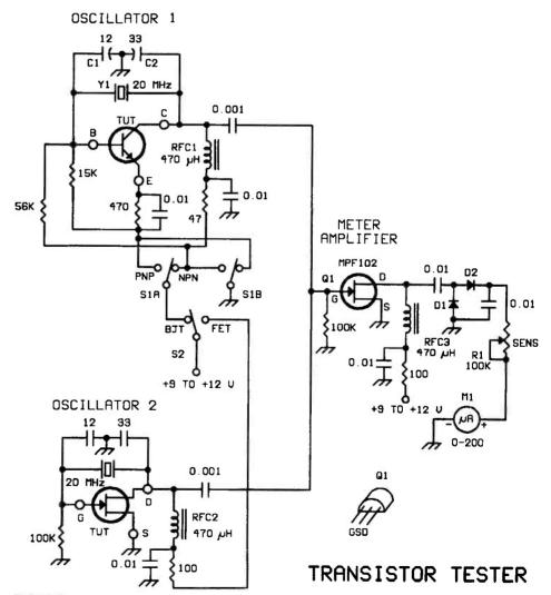
FIGURE 1 — Schematic diagram of the BJT and FET tester. Capacitors are disc ceramic. D1 and D2 are 1N60A or 1N914 small signal diodes. M1 is a surplus 100- or 200- $\mu$ A dc meter (see text). Resistors are 1/4-W carbon composition. R1 is a linear taper carbon control. RFC1 through RFC3 are miniature 470- $\mu$ H RF chokes (see text). S1 is a miniature DPDT toggle switch. S2 is a SPDT miniature toggle switch. Y1 is a surplus computer crystal.
