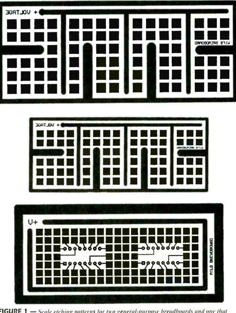
**FIGURE 1** — Scale etching patterns for two general-purpose breadboards and one that contains sites for two ICs.
