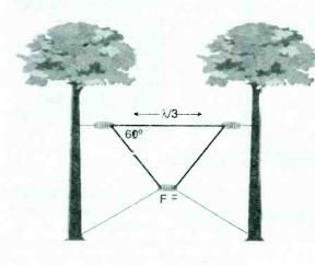
Wire is a favorite material for antennas. It is easy to work with and makes assembly and disassembly of an antenna a quick process. A onewavelength piece of wire can be used to construct a square loop antenna (above), a diamond loop (right) or a delta loop (below). The feedline attaches to the two points labeled F.
