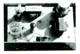
Photo of the chassis layout of the author's revised Ocean Hopper.
