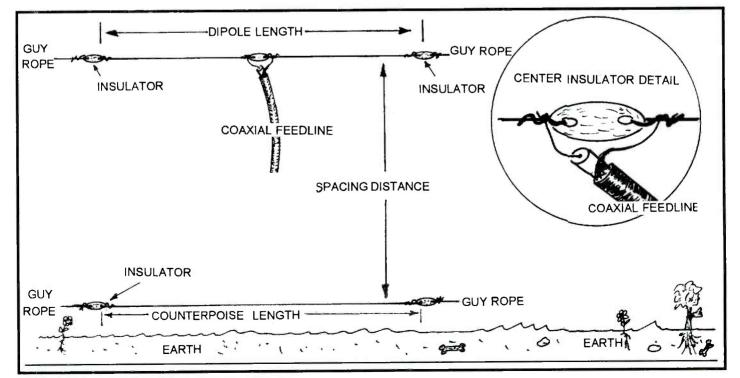
FIGURE 1. A dipole antenna with a counterpoise.
