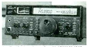
An all mode transceiver such as this ICOM IC-821H can get an amateur on all of the modes available to a Technician Class ham.
