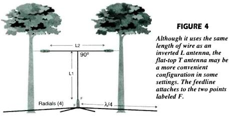
Generally, the longer the vertical section, the better the antenna performance. We used this antenna on the 41-meter band.
