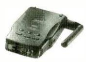
Uniden's Beartracker series is intended to provide easy access to public safety frequencies for the highway traveler. There is no frequency display, just a two-character LED to identify the state of choice and certain functional callouts. Tiny and lightweight, the units can be attached to the windshield or dash by suction cups (provided) or to the sun visor. A short swivel antenna may be removed, exposing the BNC connector which allows attachment to a cartop antenna.
