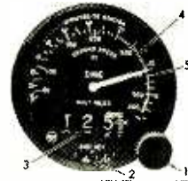
Airborne DME Distance-Groundspeed indicator display to read out the amount of flying time in minutes to or from the VORTAC station.
