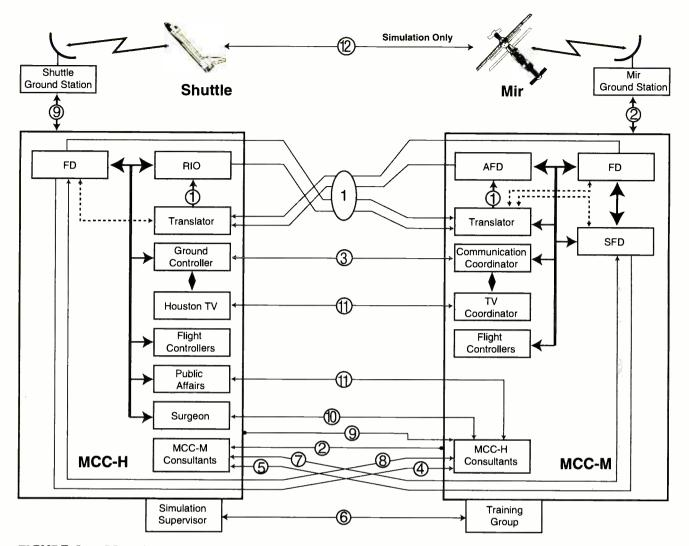
FIGURE 4: MCCs—12 communications loops interconnect the Mission Control Houston and Mission Control Moscow centers.
