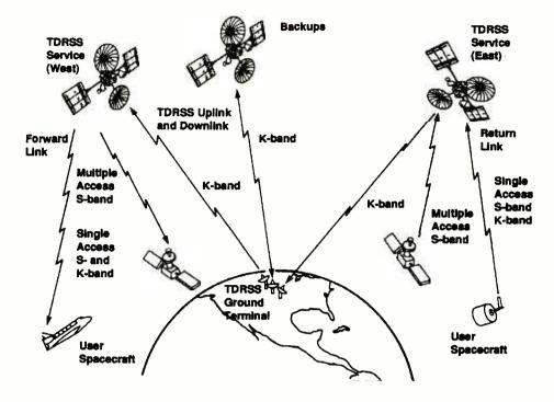
FIGURE 2: A graphic showing how TDRS is used to transmit data back to the Earth.
