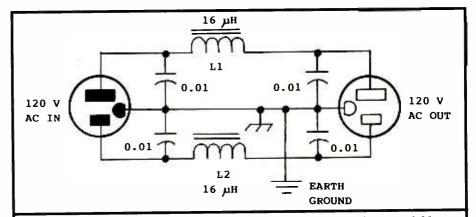
Figure 1: Schematic diagram of a brute-force line filter. Capacitors are  $0.01\mu$  at 1000 VDC. L1 and L2 have 16 turns of no. 14 enamel wire on Amidon FT-140-61 ferrite toroids. Wrap the cores with teflon pipe-joint tape (two layers) before winding the coils. You may add 150-volt MOVs (metal oxide varistor) from each side of the ac line to the filter chassis, and one MOV across the ac line, to provide spike protection for your TV and hi-fi gear.
