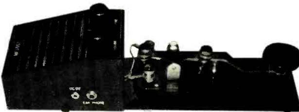
The MFJ code practice oscillator has a built-in key which, though not the best, is a very good training aide.
