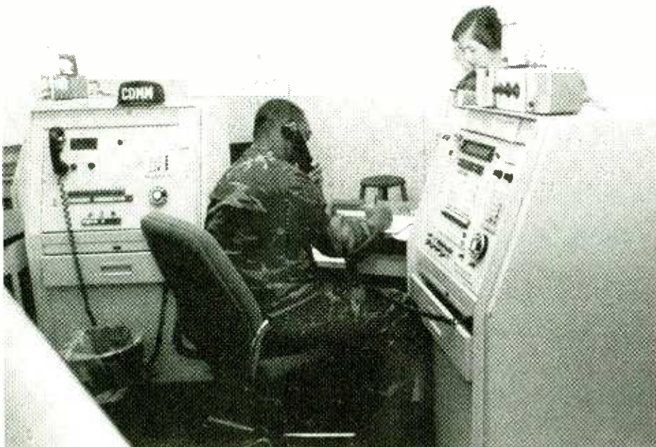
Using a SCOPE Pattern console Staff Sergeant Johnny Davis sets up a phone patch between an aircraft and a ground station. A SCOPE Pattern coordinator's console is on Davis' left.
