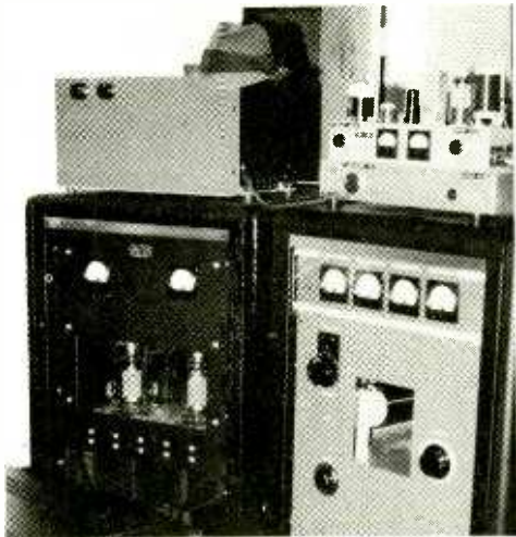
Built from scratch, the audio amplifier and plate modulator on left, exciter and power amp on right, aren't complete without Roy's hat.
