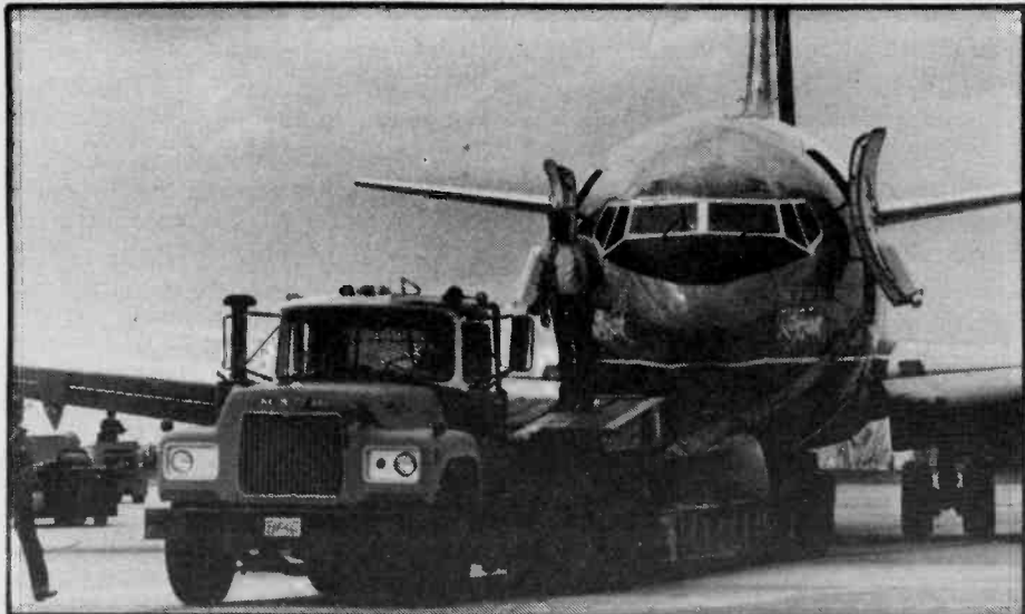
The Spirit of Kitty Hawk with its crippled front end loaded onto a flat bed trailer. This is the only way the huge airliner could be moved off the runway after it was discovered that the nose gear was destroyed.
