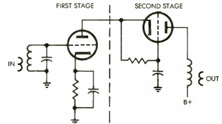
FIGURE ONE—Typical basic circuit of a cascode amplifier showing division into "stages" discussed in text. Parts values depend on tubes and frequency; Typical cathode resistor is 68 ohms. Bypasses usually are .001mF, second "stage" grid resistor 470,000 ohms.
