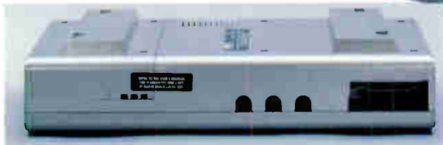
Rear outlets for power supply cords, cassette and disk drive cables.
