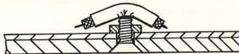
WIRE OVER SHARP OBJECT WITH PRESSURE EXERTED AND SLEEVING ON WIRE FOR PROTECTION.
