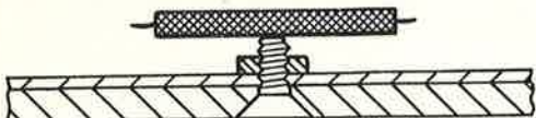
WIRE OVER SHARP OBJECT WITH NO PRESSURE BUT NO PROTECTION ON WIRE.
