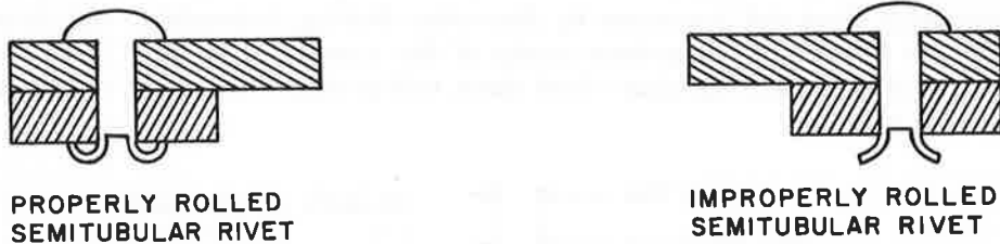
Figure 3-23. Rolled Semitubular Rivet
