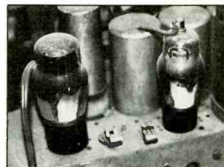
Fig. 10. Some early 1930s tubes sported a grid cap.
