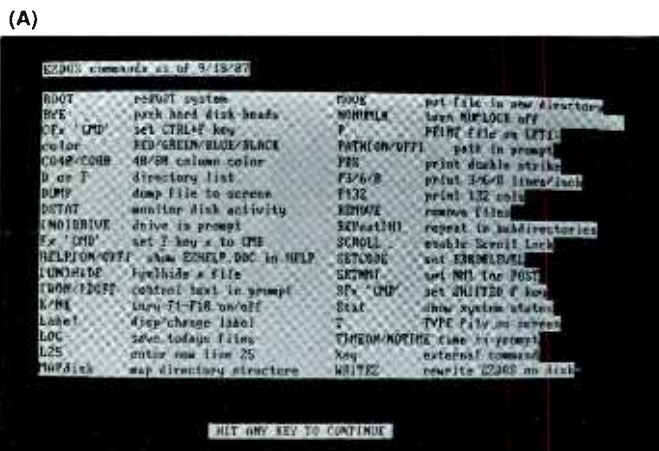
Fig. 1. Typical helpscreen of software-invoked inverse video (A) using INVERSE.BAT and ANSI.SYS and the inverter adapter. It exhibits margins at left and right of text block, with ragged right margin on unequal text lines and
