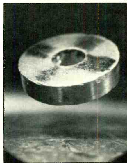
Fig. 7. The floating magnet has been pushed to one side and its rotation has stopped.
