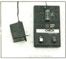
Chips to be tested plug into a ZIF (zero-insertion-force) socket to eliminate plug/unplug damage to the chip. Only two switches are provided. One turns on and off power to the instrument, while the other initiates the testing sequence. A seven-segment numeric LED display gives fast go/no-go indications, as well as automatic identification of the chip under test. Automatic current limiters prevent damage to a chip that is accidentally plugged into the ZIF socket the wrong way.
