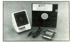
high-quality speech, sound effects and music. The computer's system unit need not be opened to install the Speech Thing, and normal printer operation is not affected. Supplied with the product is an audio amplifier with built-in speaker and headphone jack, software and manual.
