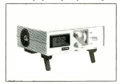
continuous from dc to 1,500 MHz (1.5 GHz) without the need for plugin elements. Power measurements are possible up to 100 watts CW or 200 watts with 50-percent duty cycle, with a resolution of 100 milliwatts. VSWR differences of 0.1 are detectable and are displayed over a range of 1:00 to 99:1. An internal 9-volt battery powers the 2.5-pound meter for up to a year. \$785.
