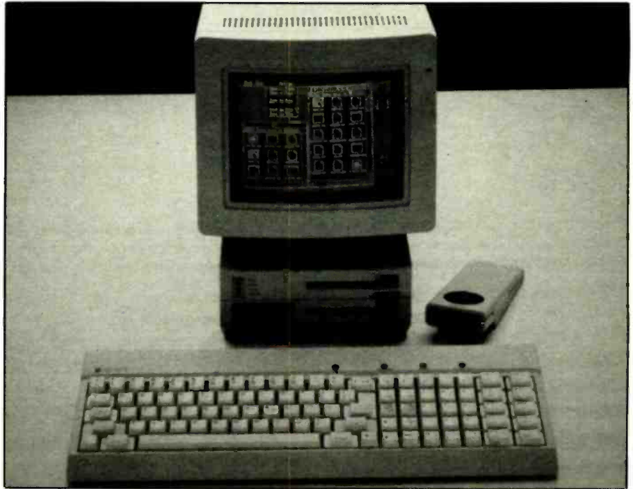
Apricot F2 features 8086 CPU, 512K of RAM, two 720K floppy-disk drives serial and parallel ports, color and monochrome interfaces and GEM software.
