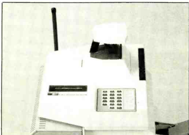
Two views of the robot's head section. Shown in the photo at the left is the hex keypad and a data/address indicator panel. Details of the status panel and top-mounted ultra-
