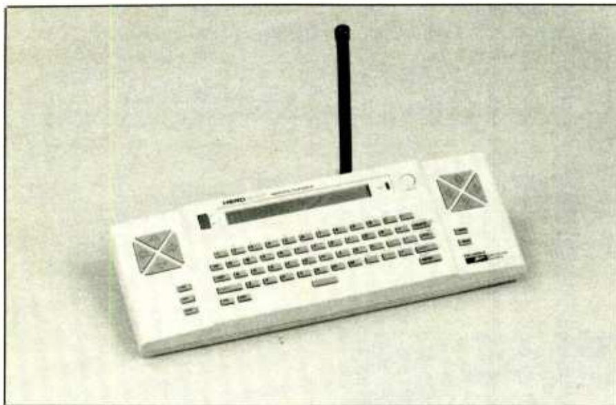
The radio-linked, 8080-based master controller has a typewriter-style keyboard, pendant controls and a 2-line LCD display panel. It has a 100-foot range.
