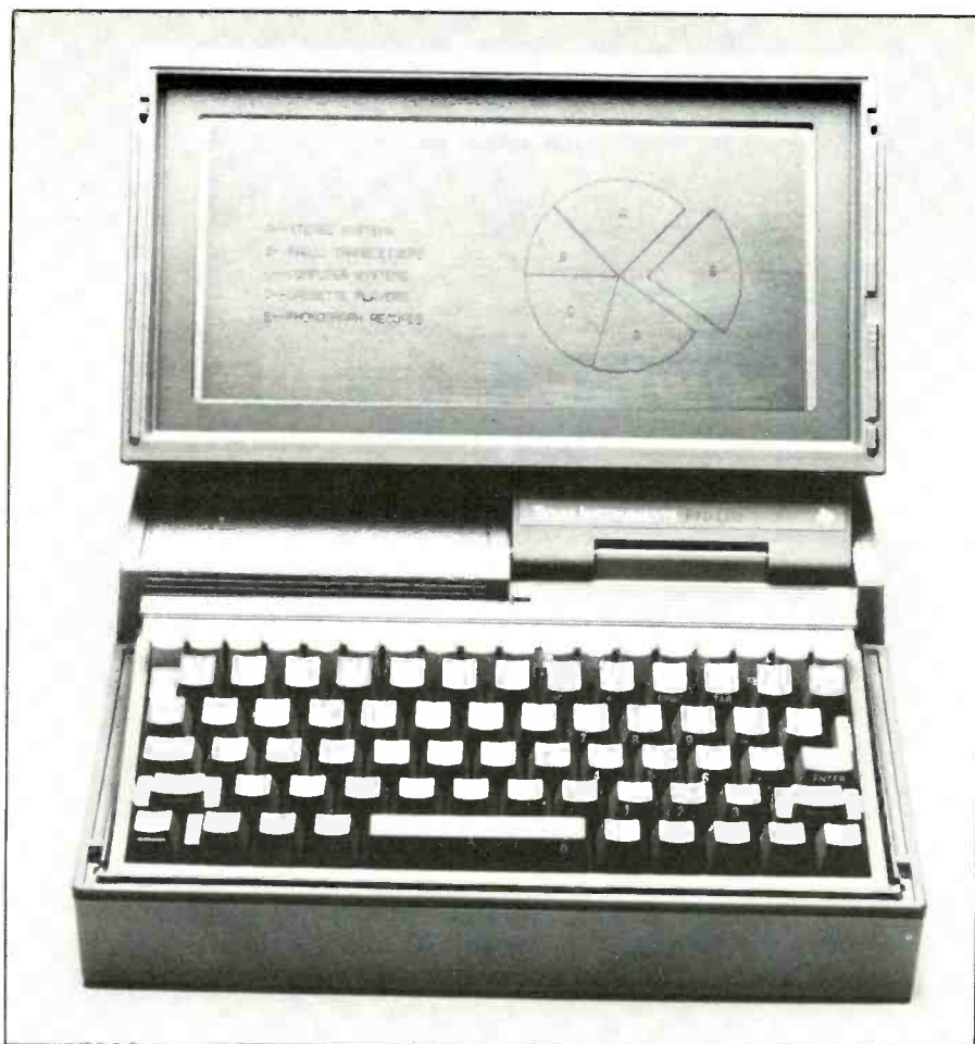
Texas Instruments' Pro-Lite features a 12" 80 × 25 LCD screen, 80C88 microprocessor, 720K of diskette storage, and user RAM expansion to 768K.
