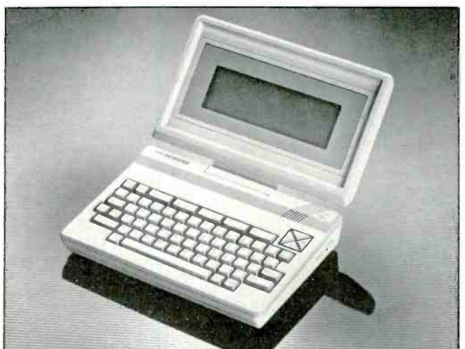
NEC's Model PC-8401A offers full 64K of RAM, built-in business software, 300-baud modem, 80 × 16 LCD screen.
