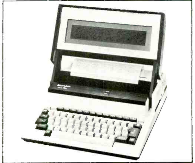
Sharp's PC-5000 provides an 80 x 25 LCD screen and a well into which you drop an optional dot-matrix printer. It uses bubble-memory cartridge, instead of disk, storage.
