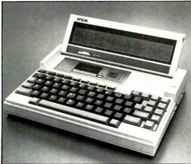
Epson's Geneva/PX-8 14-lb. notebook-size computer offers an 80 x 9 LCD screen, three applications programs in ROM, standard CP/M, 32K of ROM and 64K of RAM.
