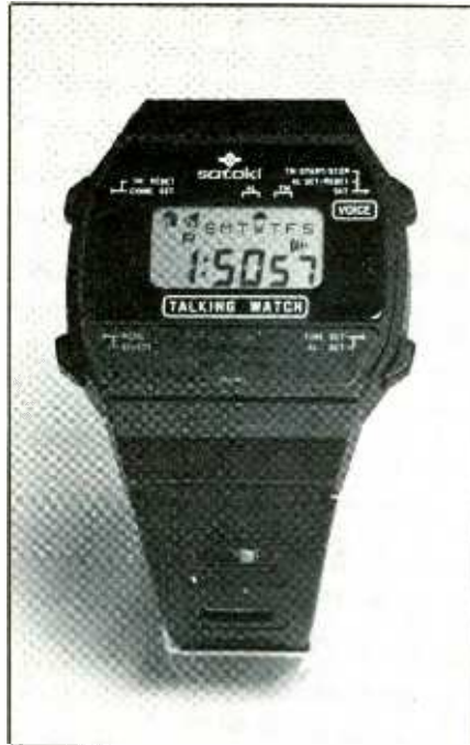
Satoki's Talking Watch backs up the usual alphanumeric display with selectable vocal announcement of time.
