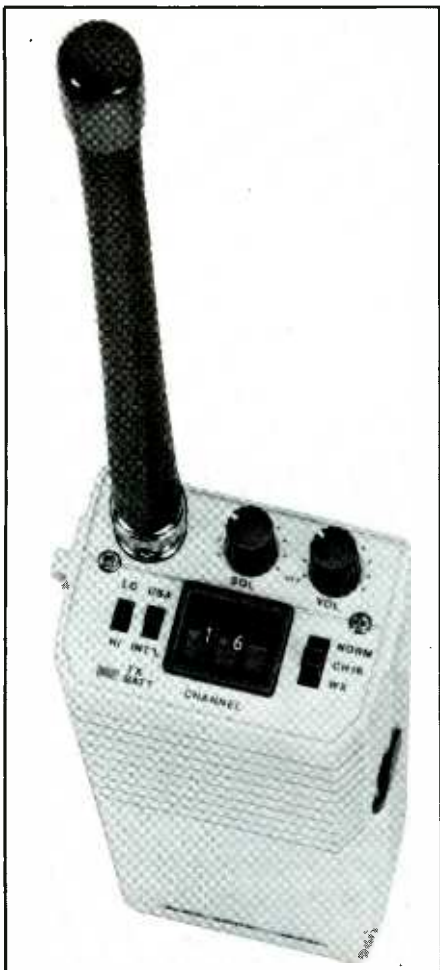
Fig. 2. Hand-held marine radios, such as the Ray Jeff model shown in this photo, offer multichannel vhf/FM communications in a convenient carry-along package.
