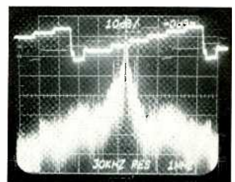
Grayscale staircase response, as indicated by the top trace in this photo, was reasonably linear in the VT-210T.
