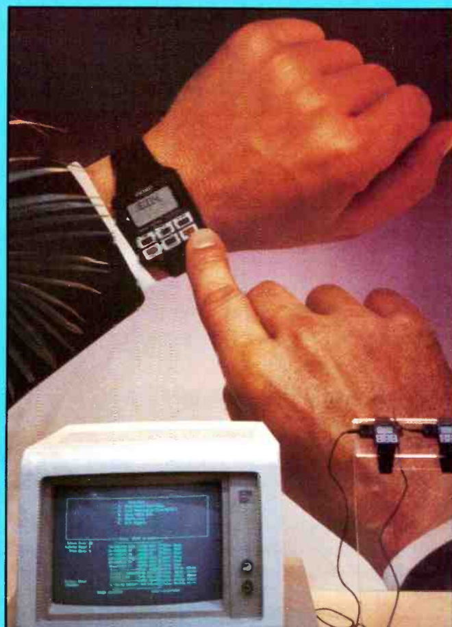
Seiko's PC Datagraph wristwatch can store up to 12 files, loaded from a computer, in its 2K of RAM memory.
