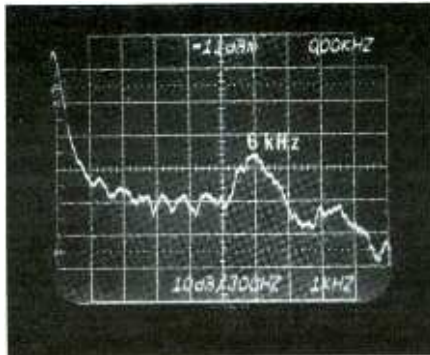
Waveform shows that speaker response is fair, except for the peak at 6 kHz.
