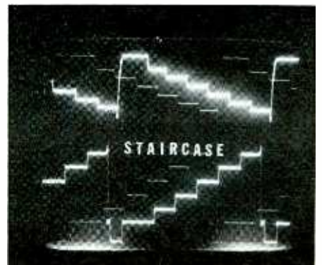
Staircase pattern at CRT (upper) and video detector reveal good grey scale.
