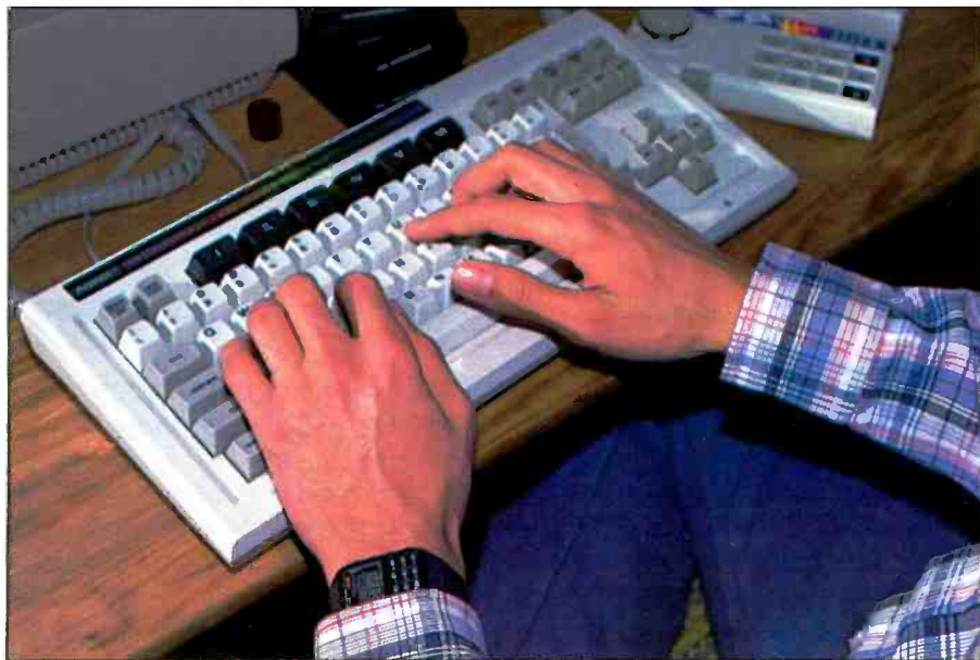
ADAM comes with a true typewriter-style keyboard with full-travel keys. The detachable keyboard can be located anywhere, limited only by its tether cable.
