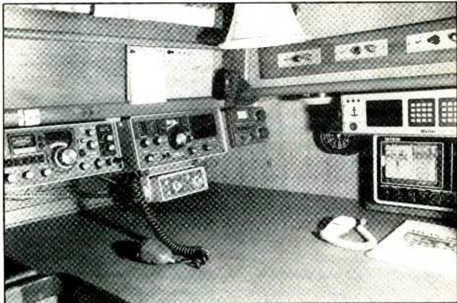
This installation shows a 350XL with a Kenwood tuner at right.
