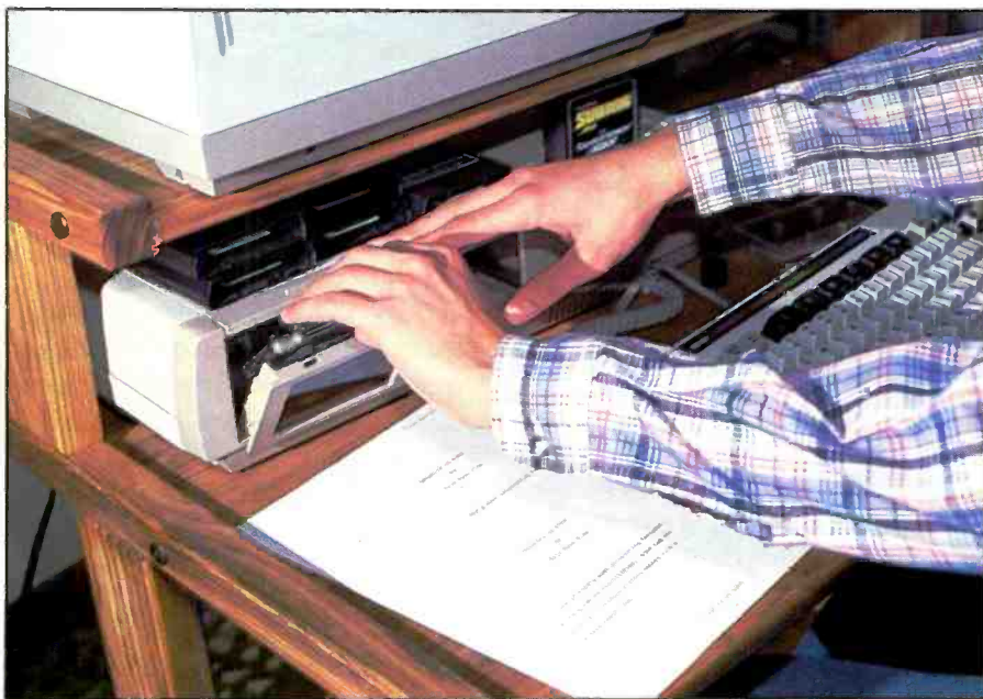
The main console easily stows under the monitor shelf on a typical computer desk as shown here. Program tapes load and unload via a flip-out cassette door.
