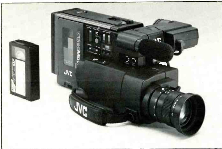
The photo above is a close-up view of the JVC Model GR-C1U video camcorder. To make the camcorder compact enough for one-hand operation (right), JVC uses a miniature version of the standard VHS videocassette (left above).
