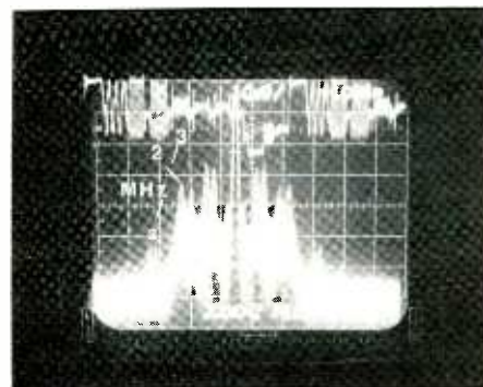
Fig. 2. This is the spectrum analyzer/oscilloscope display of multi-burst processing through the Sanyo VCR3 videocassette recorder.
