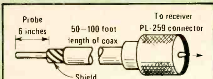
Figure 2: Try this simple rfi probe
