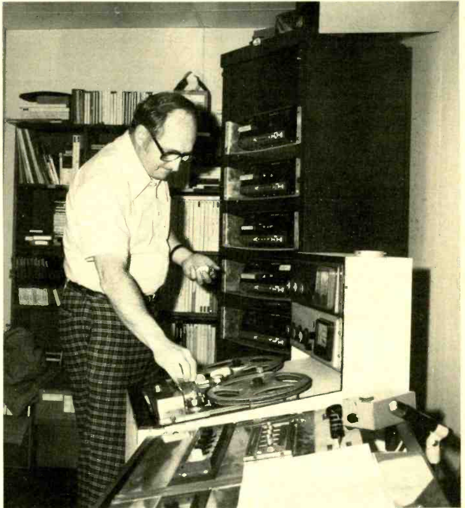
Garber adjusts one of two tape recorders in the control room of his Bellwood, PA, recording company. A custom designed sound mixing console he built is in the foreground. The large vertical equipment rack, right, contains equipment for mass duplicating cassettes. A large bookcase along the control room rear wall serves as a storage vault for several hundred master tapes and discs recorded in the studio over the years.
