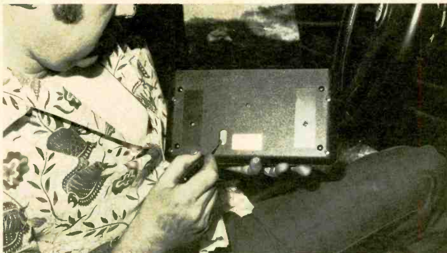
The linear tachometer, digital tachometer, and clock are programmed at a programming switch array found at the bottom of the cluster housing.
