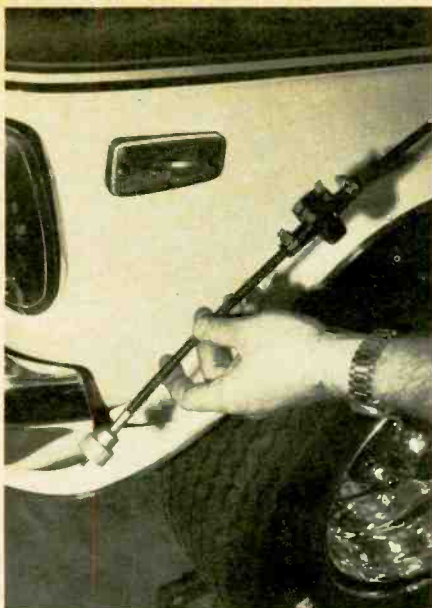
The installation directions outline how the speedo's plastic must be cut and the unique speed sensor installed in-line on the cable. The cable itself is not cut in this procedure.
