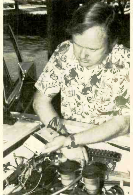
You will need two power wires for the cluster instruments: one that is hot all the time, and one that is hot only when the ignition key is turned on. Use a meter to locate the appropriate terminals for this at the fuse block.
