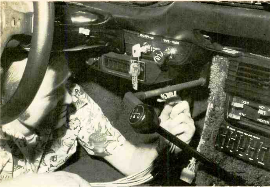
First step in the installation sequence is to route the umbilical cord up to the top of the dash where the housing will be located. Next, run the wiring harness through the car's firewall and into the engine compartment.
