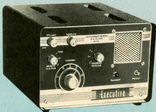
International Crystal Manufacturing Co., produced an extensive line of Executive model transceivers, all quite popular. This was the set by the time CB had grown to the point where operators wanted operating capabilities extending past "single channel" rigs. This set offered 3 transmit channels and a tunable receiver, plus 3 crystal controlled receive positions.
