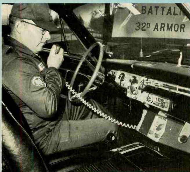
It wasn't that tube-type CB rigs weren't good pieces of electronic equipment, but they did tend to become a bit bulky when mounted in mobile units.
