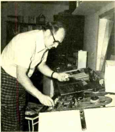
Asbury Recording Company owner Earl Garber uses a stop watch to accurately time a segment from a master tape playing on one of two stereo recorders in the control room. Exact timing is essential so a selection will fit on a disc or tape cassette. The master mixing and control panel is at Garbers left.
