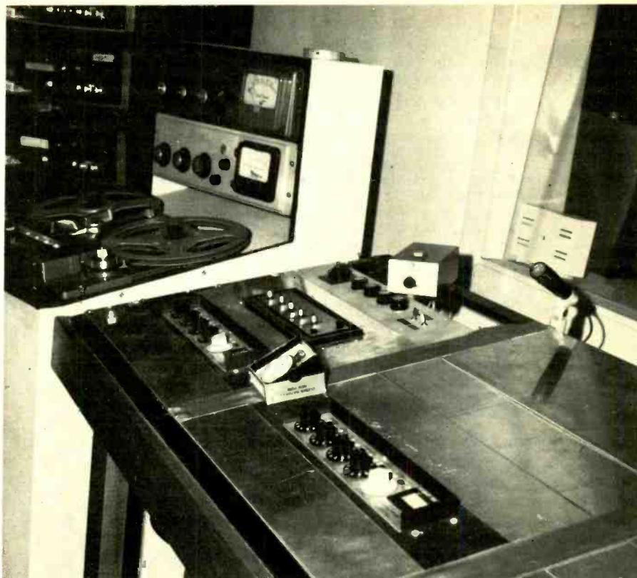
Closeup view of Asbury Recording Company master control and sound mixing console in the foreground. Eight separate microphone inputs can be feed to two professional stereo tape recorders either individually or combined. A Crown stereo professional tape recorder sits to the left of the master console. The microphone near the top of the control panel is used for control room-studio talk back communications.
