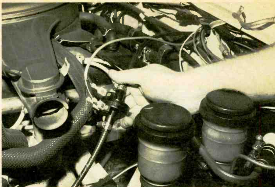
Certain wires from the wiring harness are then connected to the terminals on the speedometer sensor. Again, plastic insulated connectors are utilized.
