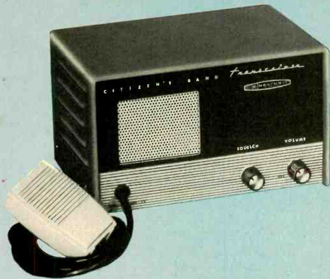
The Heath GW-12 was an early kit, in the days when the FCC allowed CB'ers to build their own sets. A single channel rig, it did a most respectable job.
