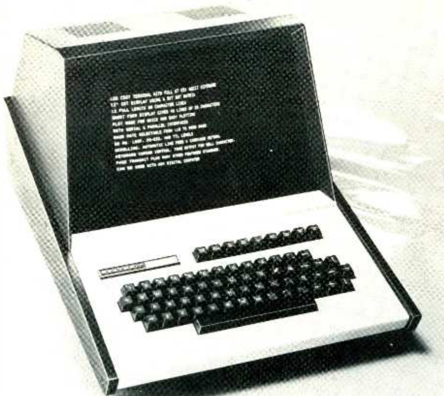
Heathkit's model H9 cathode-ray tube (CRT) terminal includes a keyboard so you can send commands and requests for action into the computer and a video-display tube so it can send out its answers.
