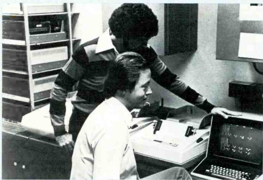
Members of Knott's Berry Farm construction and maintenance division check operations on one of their three MITS home-style microcomputers. Left of the CRT (cathode-ray tube) keyboard and video-display terminal are paper printers. The actual computers are at far left. These are the same microprocessors home-computer hobbyists use.
