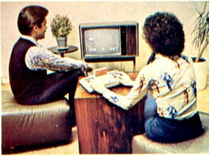
RCA's Studio II programmable video game uses a calculator-like keyboard to control the action.
