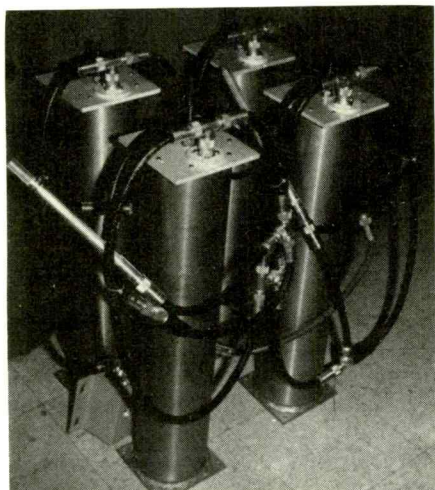
Duplexers are machined metal tubes, or "cavities," which allow use of a single antenna for transmitter and receiver.
