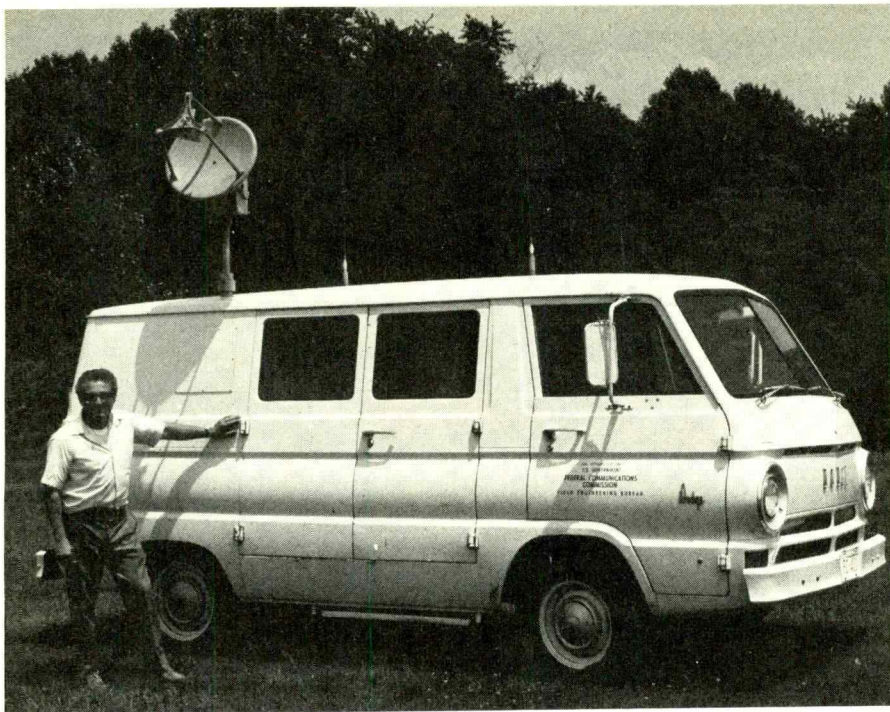
Most CBers picture the FCC using vans like this in their CB enforcement effort. Actually, these vans are used to monitor microwave transmissions such as those made by the telephone company and other common carriers. The SEF engineers use ordinary four-door sedans.
