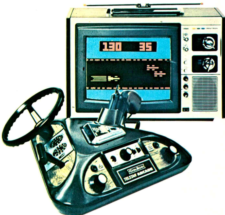
The Coleco Telstar Arcade, although offering the fewest games of any programmable set, gives you greater feel for the game by providing realistic control action. Instead of turning a rotary control, or moving a joystick, you steer your racecar with a real steering wheel, and shift gears with a separate shift lever.
