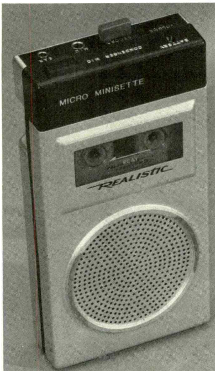
Realistic model 14-814 Micro Miniset from Radio Shack has low-battery LED tattletale, weighs 12 ounces. Shirt-pocket General Electric model 3-5330 Micro II, top of this page, has one-button operation, end of tape signal.
