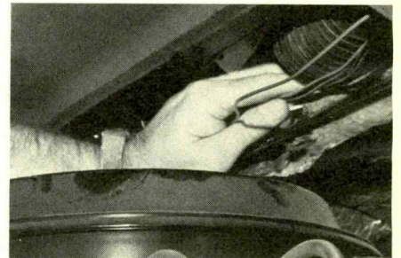
First step is to locate an out-of-view mounting location for the alarm module, which we determined to be behind the dashboard in front of the passenger's seat. The wiring harness was located at this point and its wires routed to various locations as needed.
