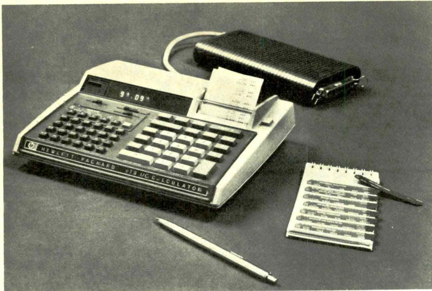
Is it a calculator or a computer? The model 97S input and output (I/O) calculator by Hewlett-Packard is a "computing data acquisition device" that combines the HP-97 portable programmable calculator with computer-like BCD interfacing to make a low-priced machine for instrument data collection and computer applications.
