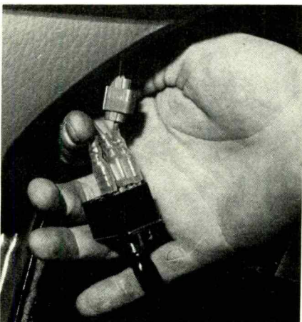
Remove the antenna's control switch from the dash and tie in the wire from the transmitter with a connector.
