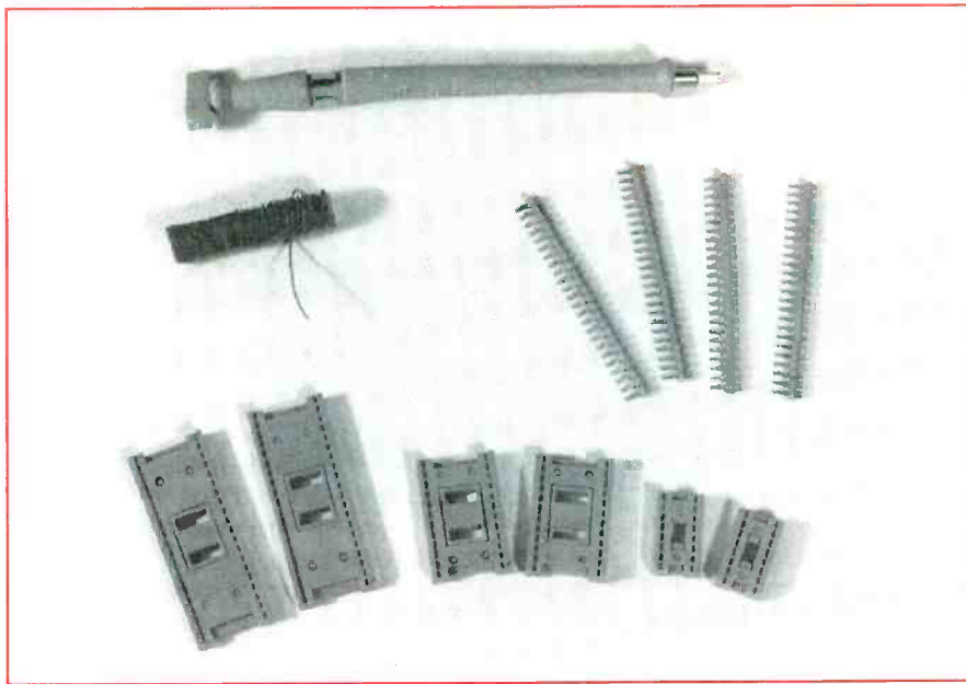
Fig. 10. Materials for Scotchflex breadboarding. Clockwise from top: universal tool, plug strips, dual sockets, wire.
