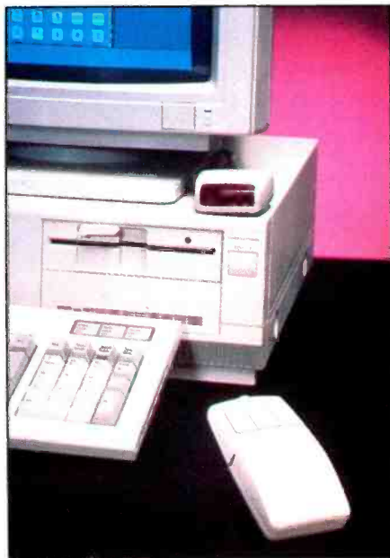
Fig. 1. The Cordless Mouse operates over a range of up to 5 feet between mouse transmitter and receiver and up to 90° off-axis over an infrared link.
