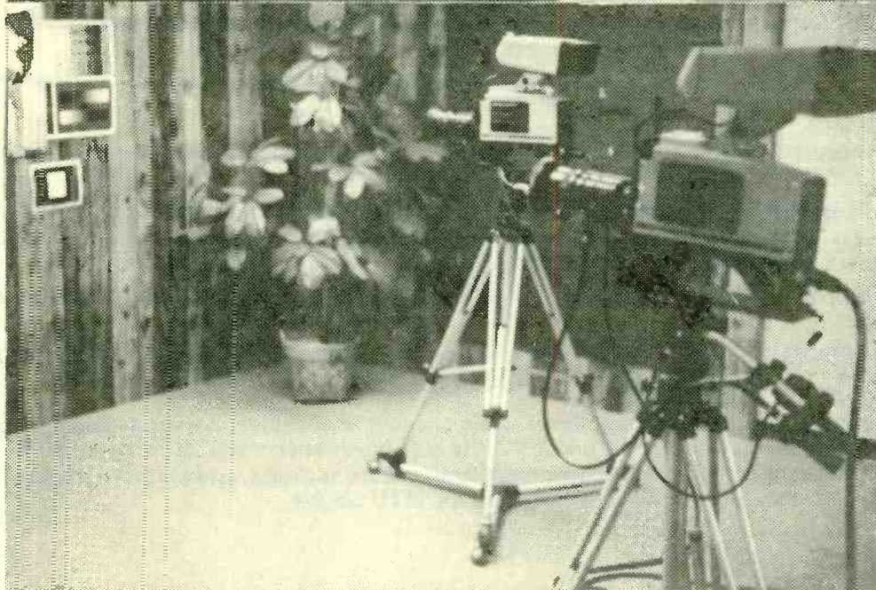
Left: Two Panasonic WV 7700-3 tube prism cameras with studio viewers are used.
