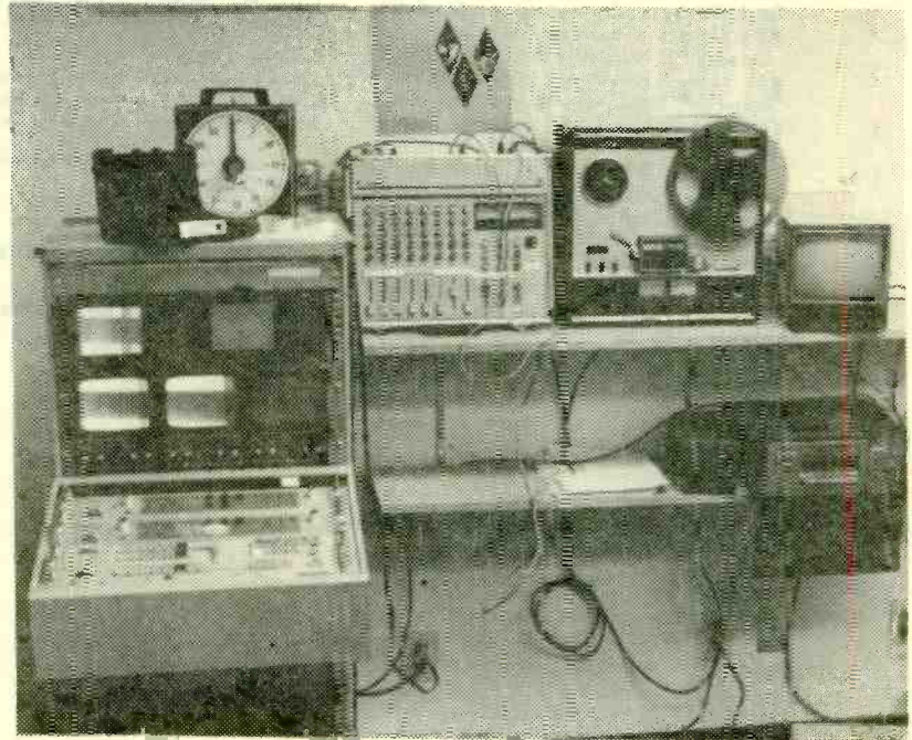
Switcher and monitors on rollable dolly can leave the control room for use on remotes.
