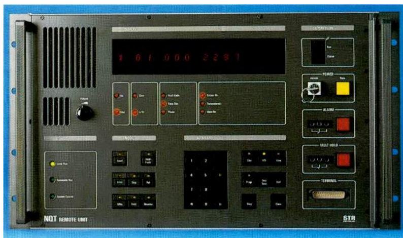
Operator panel of the exchange-based test unit.
