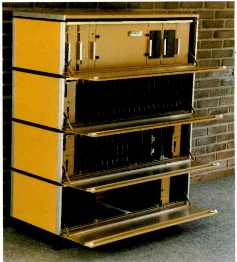
Databocs shelf stack, showing the PABX shelves and microprocessor shelf.
