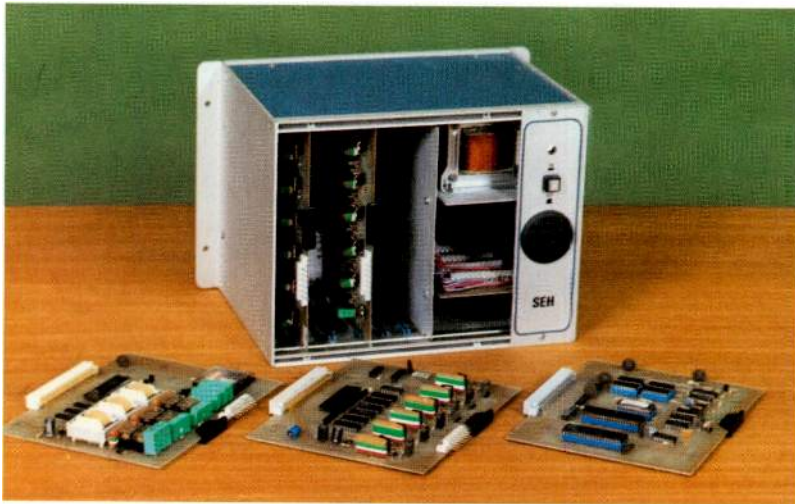
PABX with the exchange line, extension line, and central processor boards removed.
