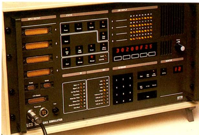
Front panel of the STR local call simulator.
