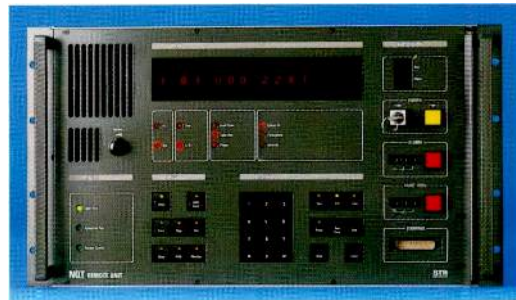
A network quality tester remote unit.
