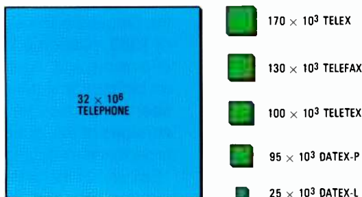
Figure 2 Number of subscribers expected to use the main narrowband services in the Federal Republic of Germany in 1990.
