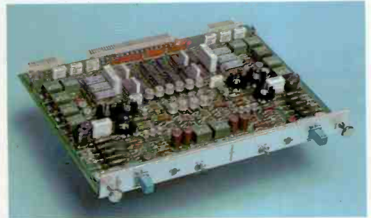
Printed board for the Unlink signaling converter.
