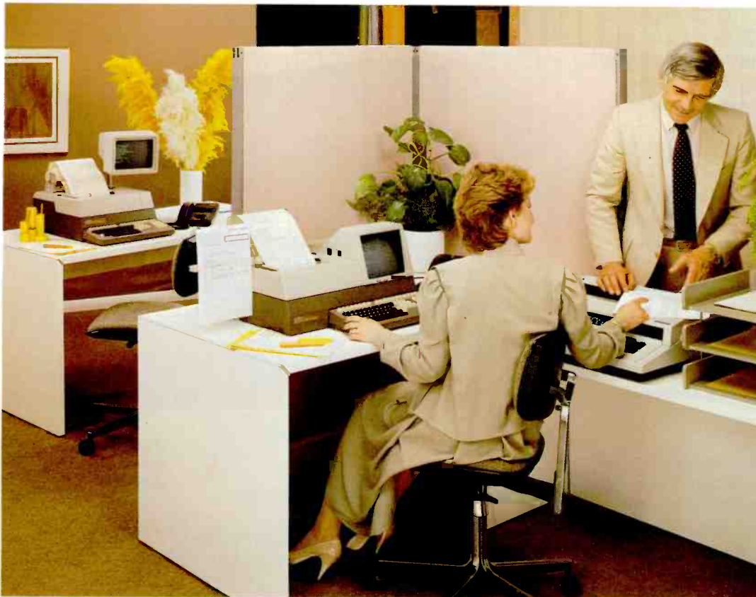
ITT3000 teleprinters. The modular version is to the left and the integrated version in the center.
