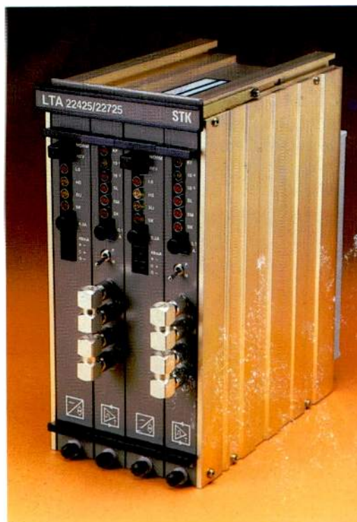
Line terminating assembly for STK's 10-channel PCM system.
