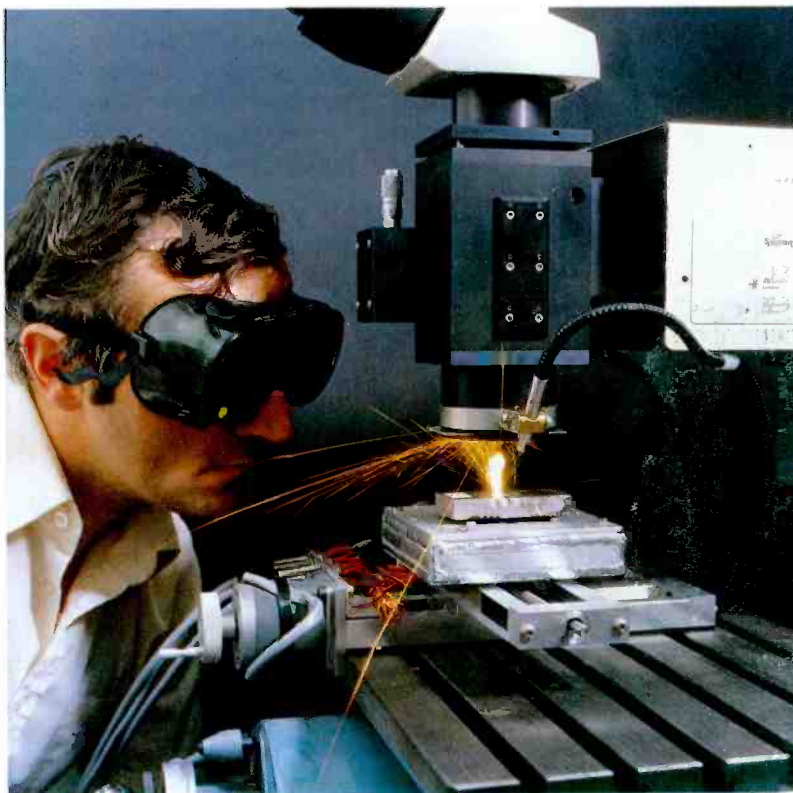
Automatic machining of ceramic using an Nd/YAG laser.
