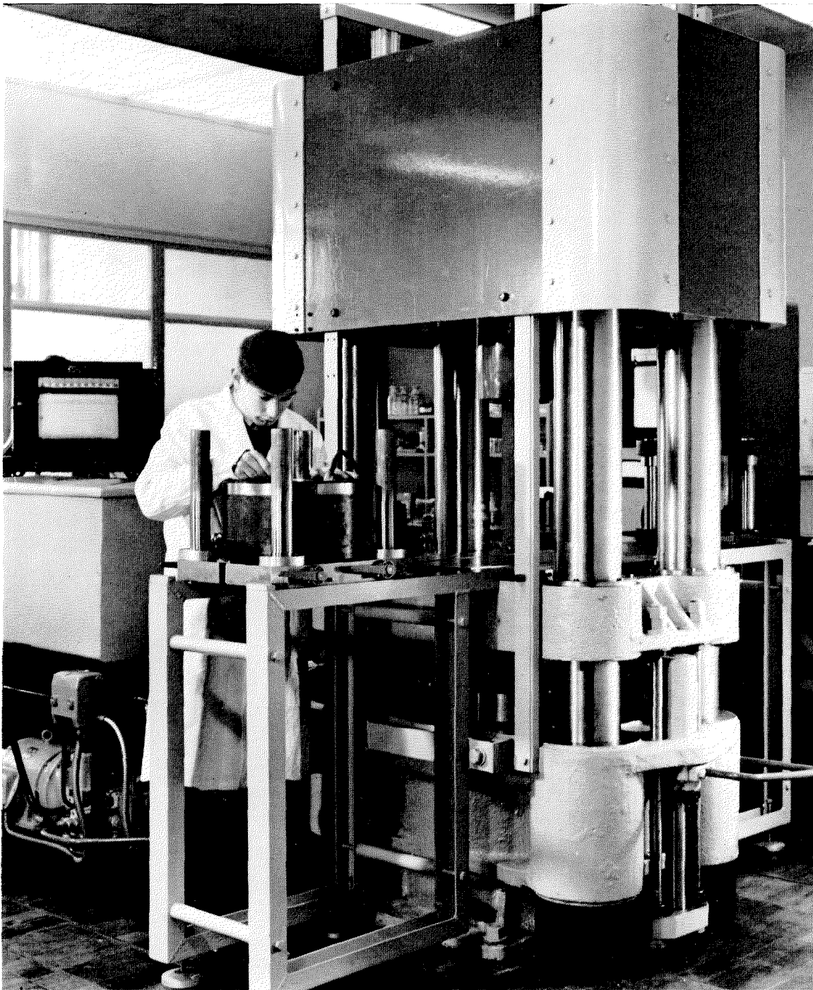
Figure 9—A machine which can apply pressures of more than 100 000 atmospheres, or 1.5 million pounds per square inch (105 megagrammes per square centimetre) to a sample of material, which can be heated simultaneously to 2000 degrees centigrade. The aim is to produce new materials with improved properties which may be useful in new types of transistors or insulators.
