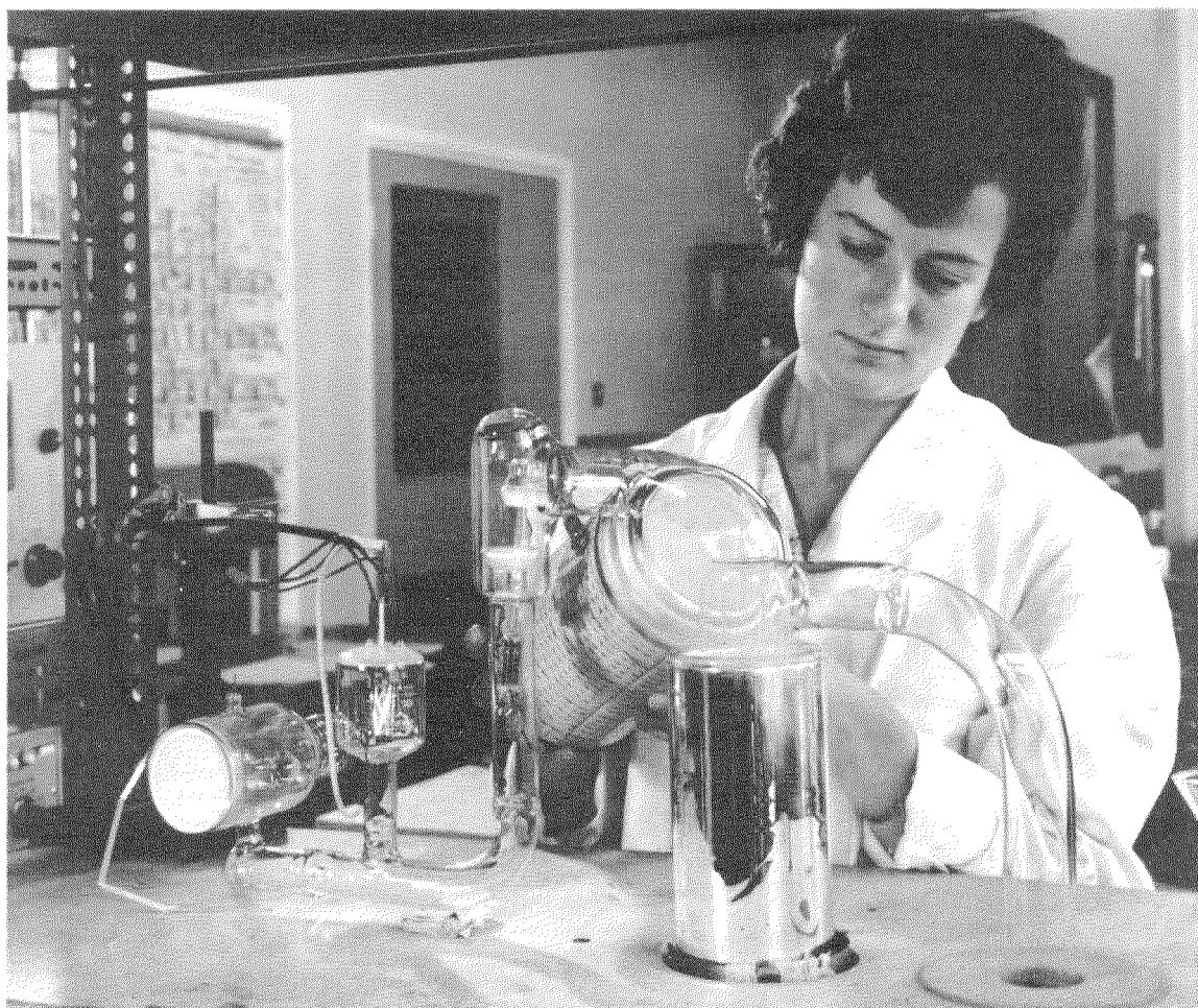
Figure 11—A field-emission microscope used in the study of semiconductor surfaces. This equipment enables an image of the surface of a fine point of the material under investigation, magnified some 100 000 times, to be observed on the fluorescent screen (seen on the extreme left). The liquid air being poured into the Dewar flask is to maintain an ultra-high vacuum ( 10^{-9} torr) within the system. The glass-work is of special construction required for ultra-high-vacuum studies.
