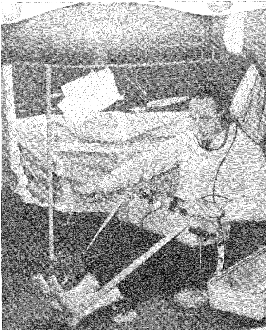
Figure 4—Operation of lifeboat rescue radio set.
