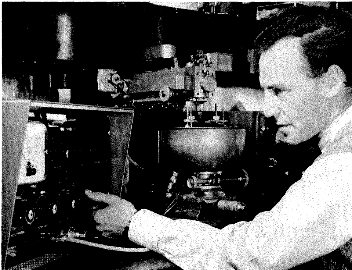
Figure 12—Equipment for machining to extremely close tolerances by spark erosion, built as a research tool to facilitate a study of the physics of erosion and to establish the ultimate limitations of the process. Individual spark discharges, occurring at high frequency, remove micron-size particles without physical contact between the electrode and workpiece contained in the bowl. The machine is being used in the construction of millimetre-wave tubes and components, thin-film evaporation masks for microcircuits, and the direct machining of semiconductor materials. Results obtained would not be possible by any other means.
