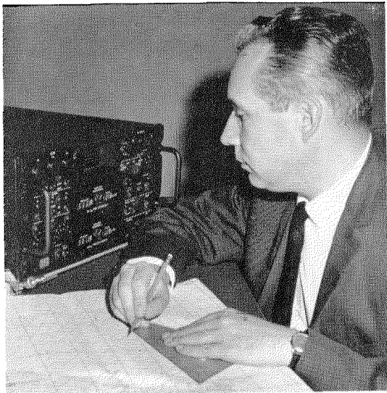
Figure 7—Self-tracking low-frequency loran receiver providing continuous precise position data out to 1500 miles (2778 kilometers).
