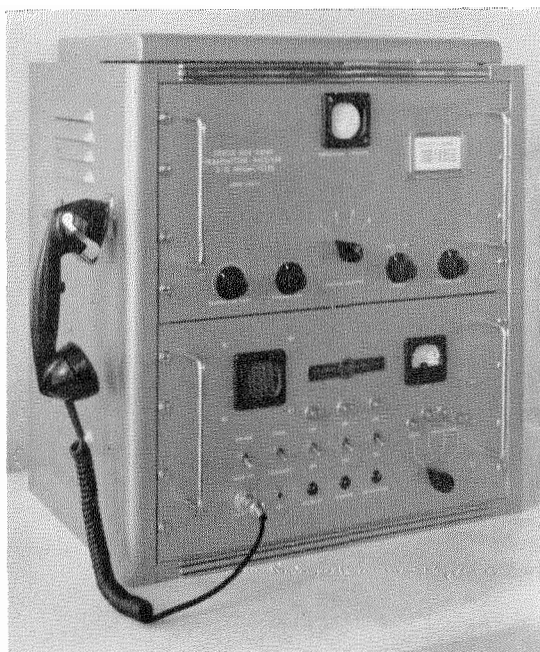
Figure 13—Marine radio receiver, which covers from 70 kilocycles per second to 30 megacycles per second.
