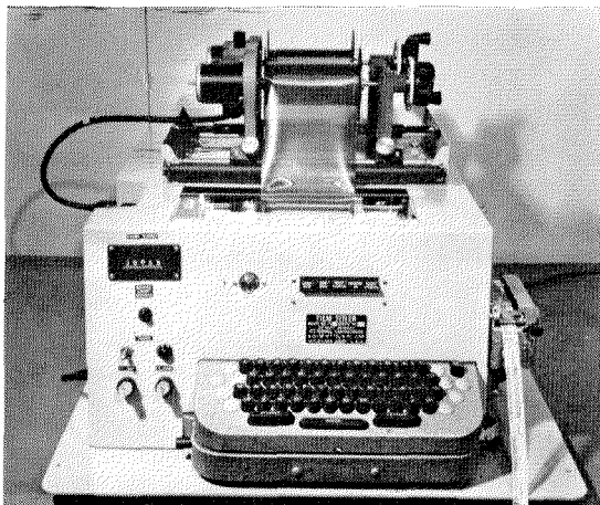
Figure 3—Film titler permits single manual typing of a caption or its repetition under control of a paper tape.
