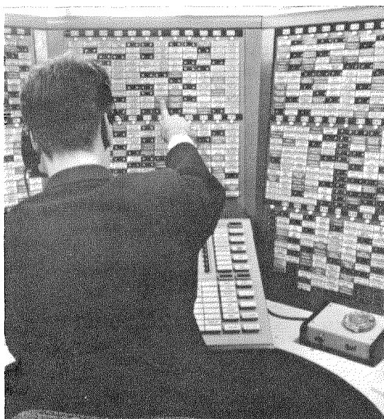
Figure 2—Part of the Doris console for the Direct Order Recording and Invoicing System utilizing pre-recorded data and punched tape for the full processing of orders.
