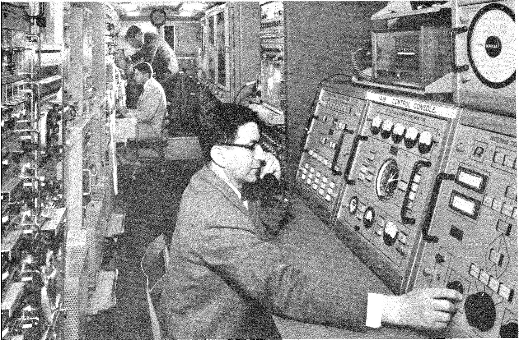
Figure 1—Courier satellite ground equipment for handling 340 000 words to and from the satellite during its 5-minute exposure to the ground station on each trip around the earth.
