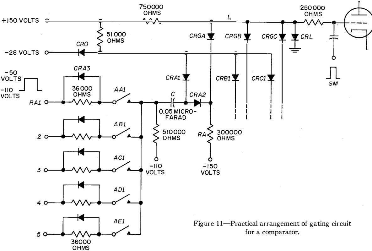
Figure 11—Practical arrangement of gating circuit for a comparator.
