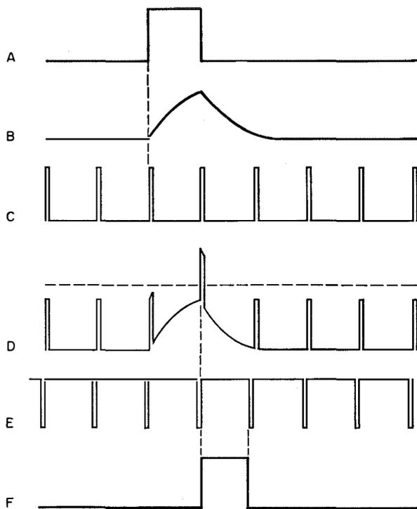
Figure 2—The original pulse at *A* is distorted by filtering action to the shape shown at *B*. *C* are start marker pulses, one of which is lifted at *D* by the distorted pulse of *B*. The lifted pulse triggers the regenerator which produces a new clean pulse *F* until it is stopped by the reset marker pulse at *E*. The new pulse is exactly one interval later than the original pulse.
