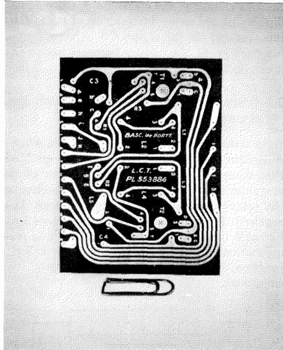
Figure 12—Rear of flip-flop panel.
