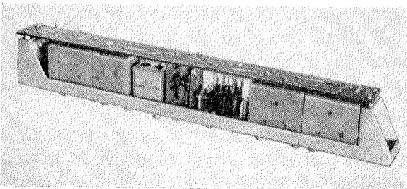
Figure 17—Line circuit including the magnetic amplifier for ringing.
