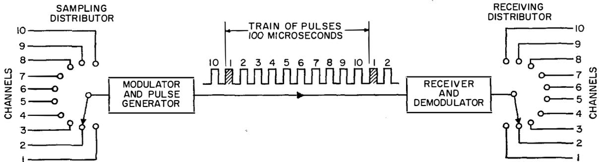
Figure 7—Principle of a time-division multiplex system.
