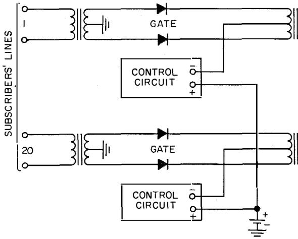
Figure 7—Method whereby individual control circuits can make the gate of a subscriber's line conductive by reversing the polarity of and exceeding the voltage supplied from a common battery that normally holds the diodes in blocking condition.
