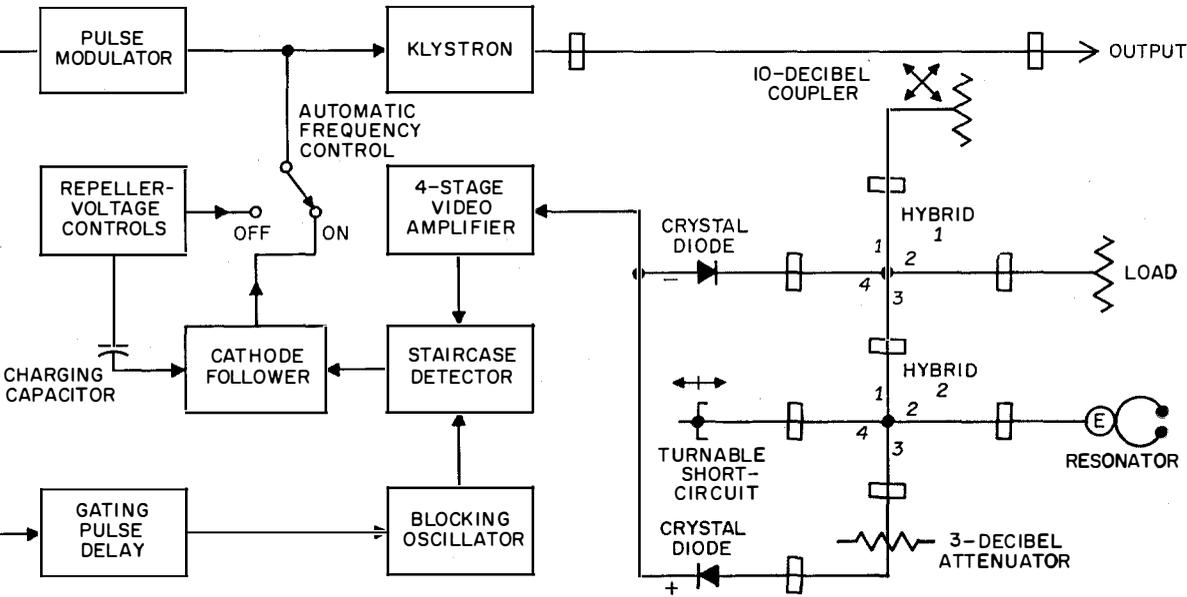
Figure 1—Block diagram of automatic-frequency-control system.
