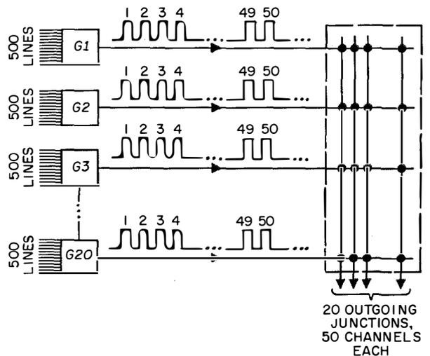
Figure 8—Combination of time switching with space switching.
