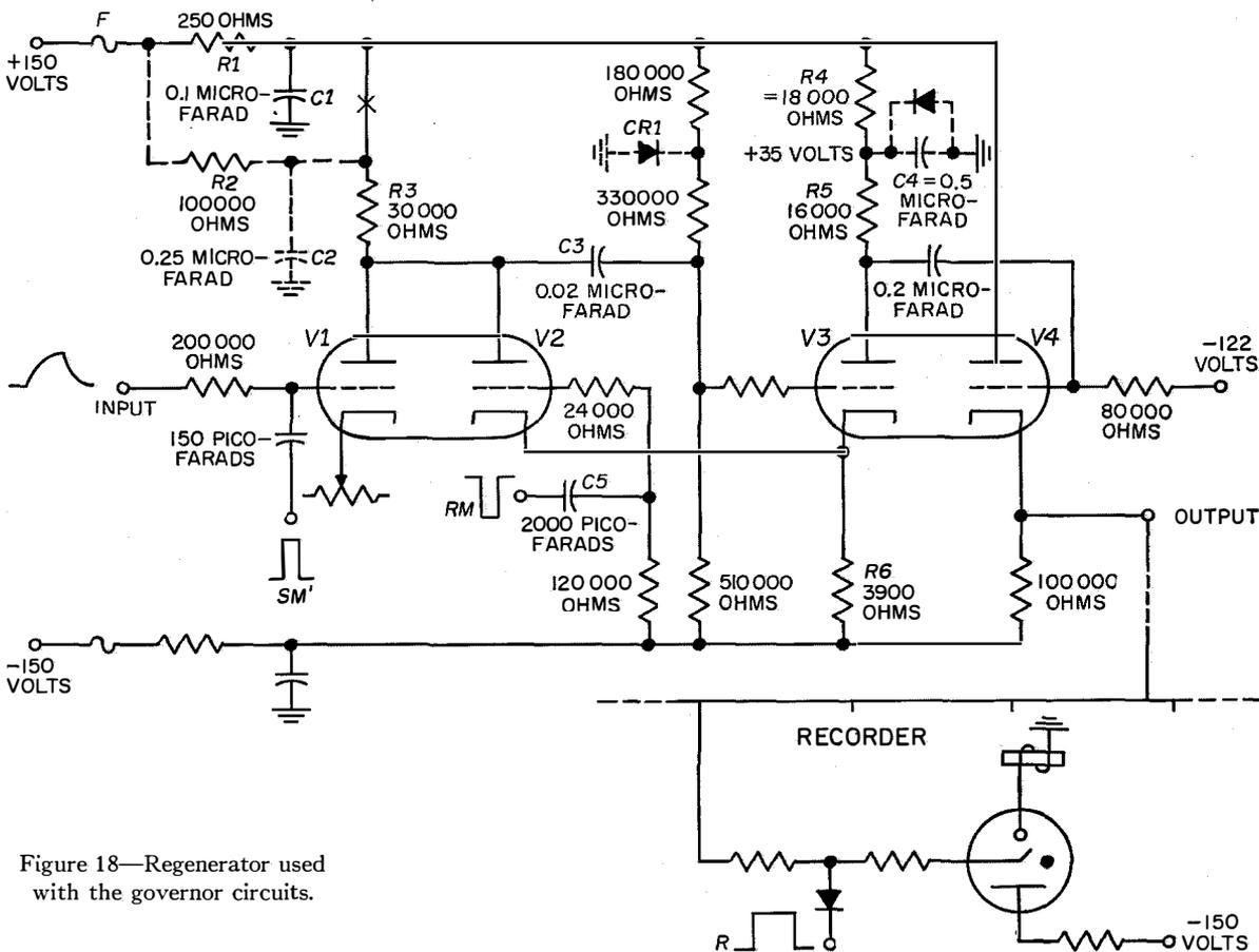
Figure 18—Regenerator used with the governor circuits.
