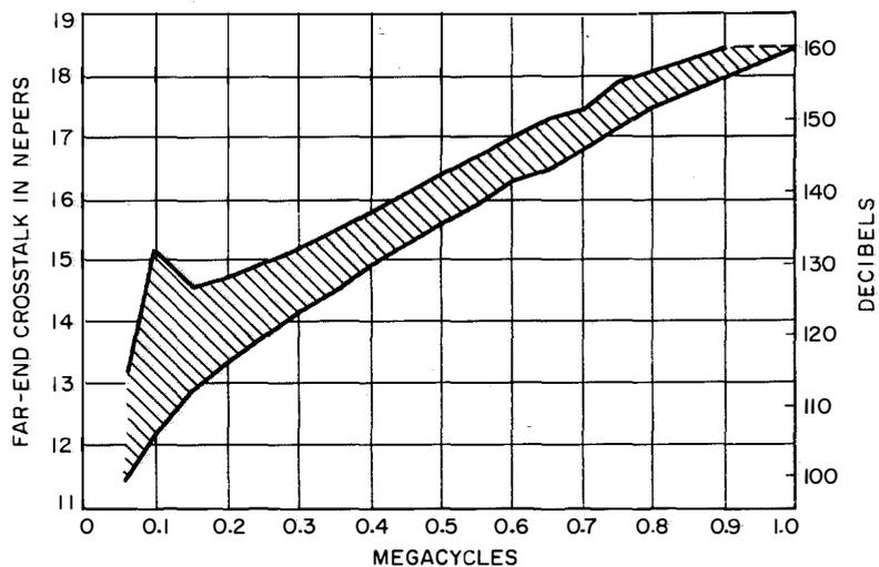
between these circuits. Typical results are shown in Figure 13 for near-end crosstalk and in Figure 12 for far-end crosstalk.
