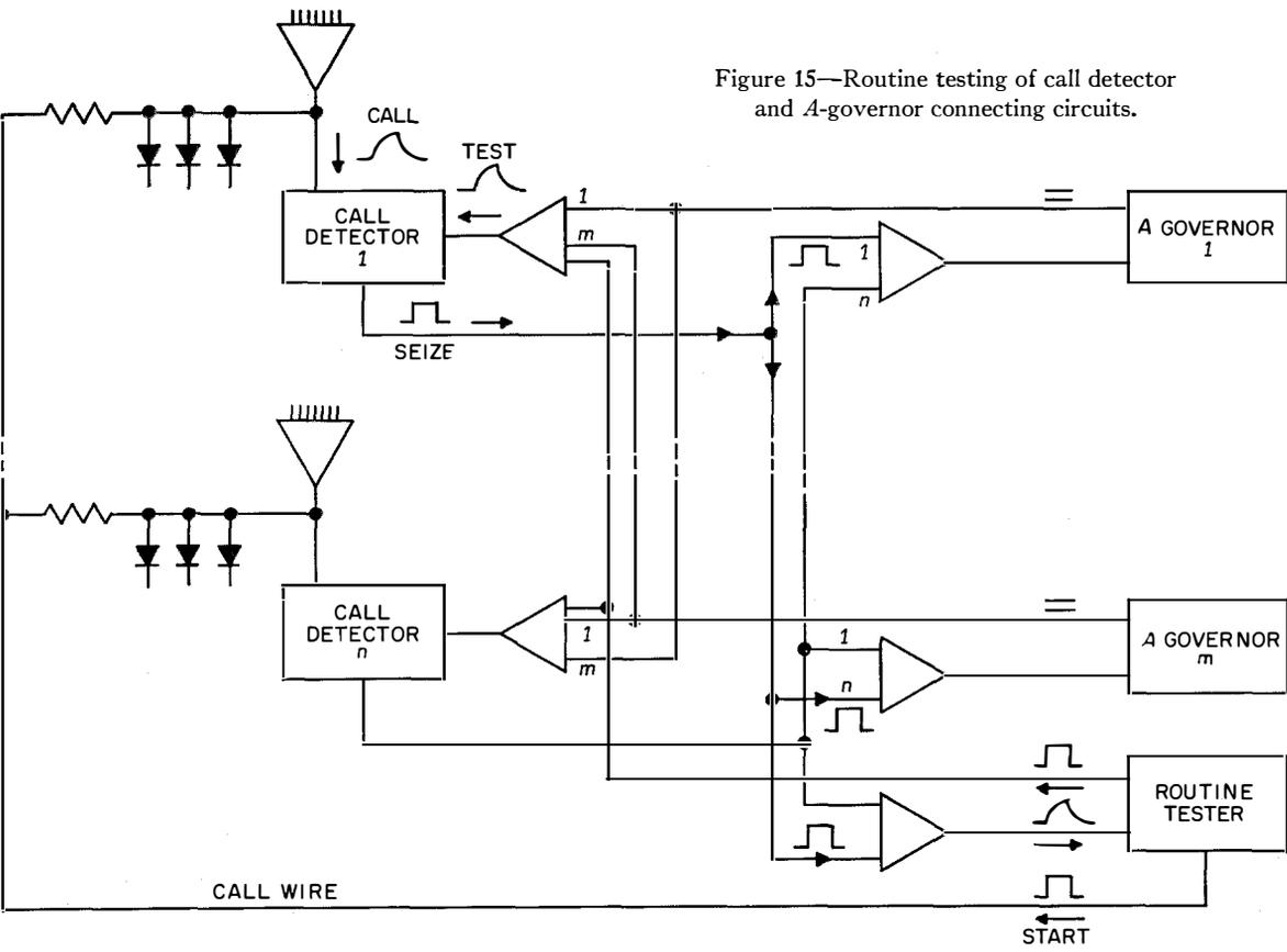
Figure 15—Routine testing of call detector and *A*-governor connecting circuits.
