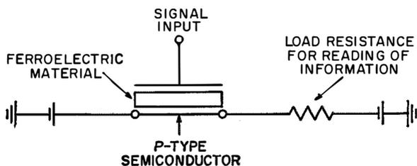
between the electrodes. This electrode may be a semiconductor containing impurities of the *P* type. With this type of storage, conductor current through the semiconductor electrode will permit the reading of information from the capacitor store.
