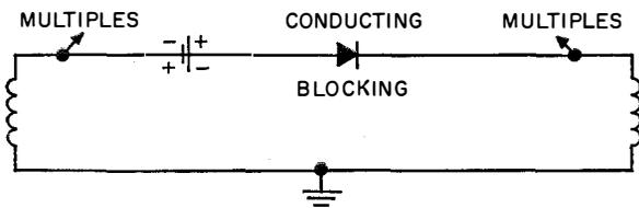
Figure 3—Diode and biasing battery connected between windings of two transformers to act as an opened or closed switch depending on the battery polarity.
