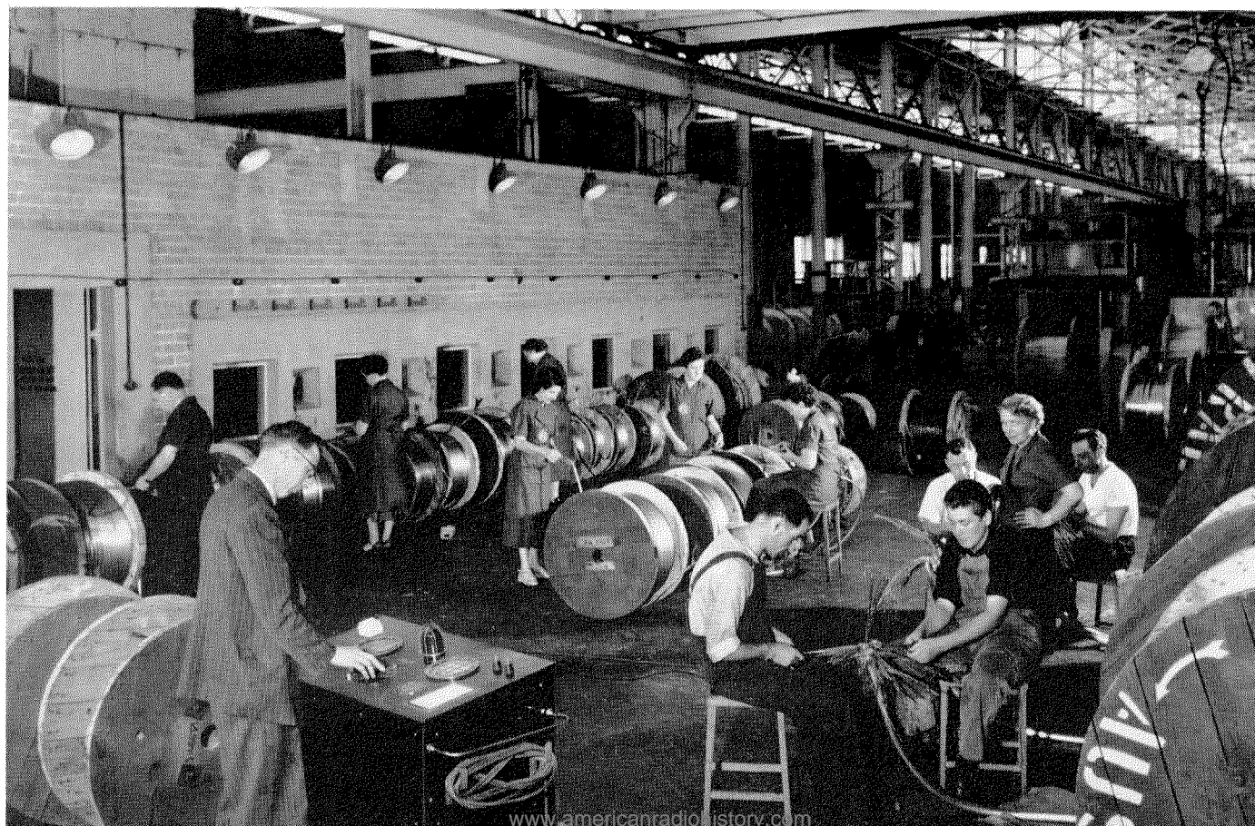
14. On this page are shown the testing of completed cable ends and above is the alternating-current test room where cable frequency characteristics are checked.
