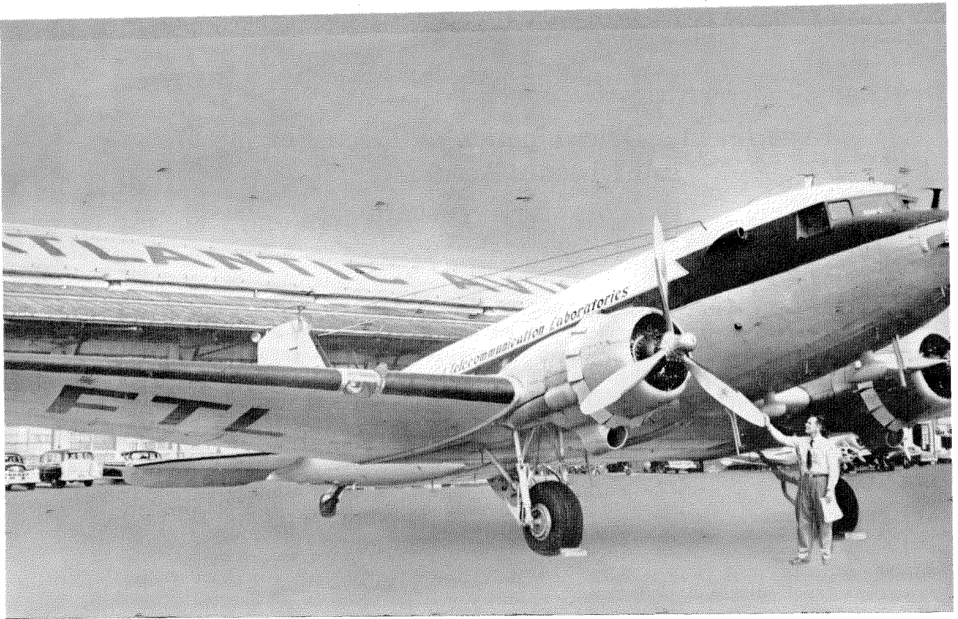
Figure 1—The DC-3 "flying laboratory" used in tacan accuracy-determination flights.
