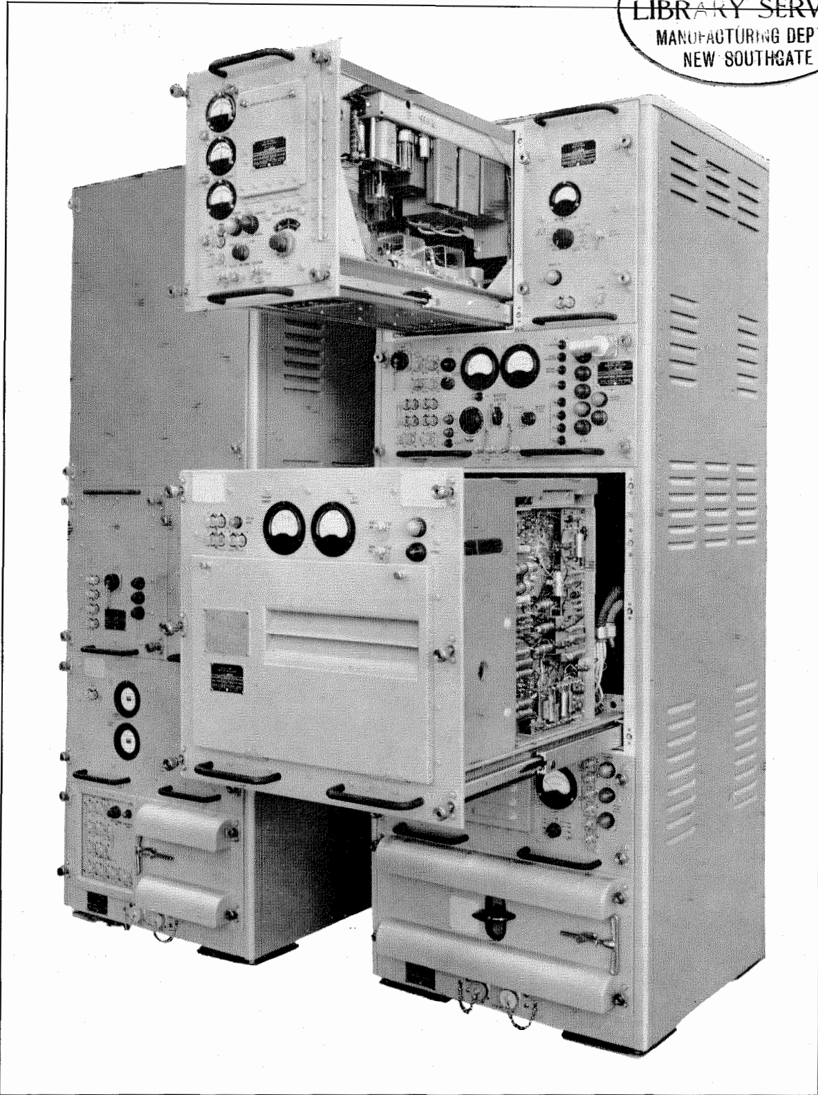
Figure 2—Two of the slide-mounted drawers pulled out fully to demonstrate the accessibility provided by the design.
