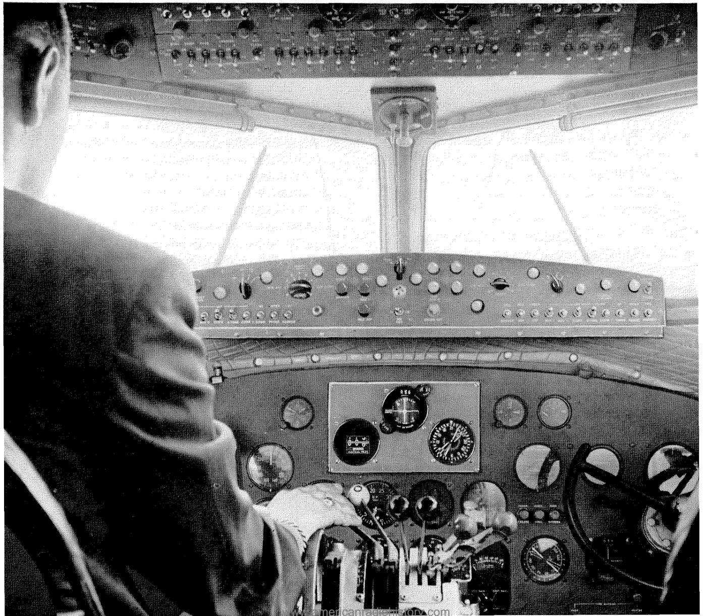
Figure 3—In the pilot's compartment, the left meter gives distance and the center and right meters give bearing.
