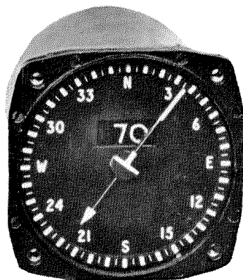
The airborne indicator gives bearing by a pointer and distance by a number display on a single instrument.
