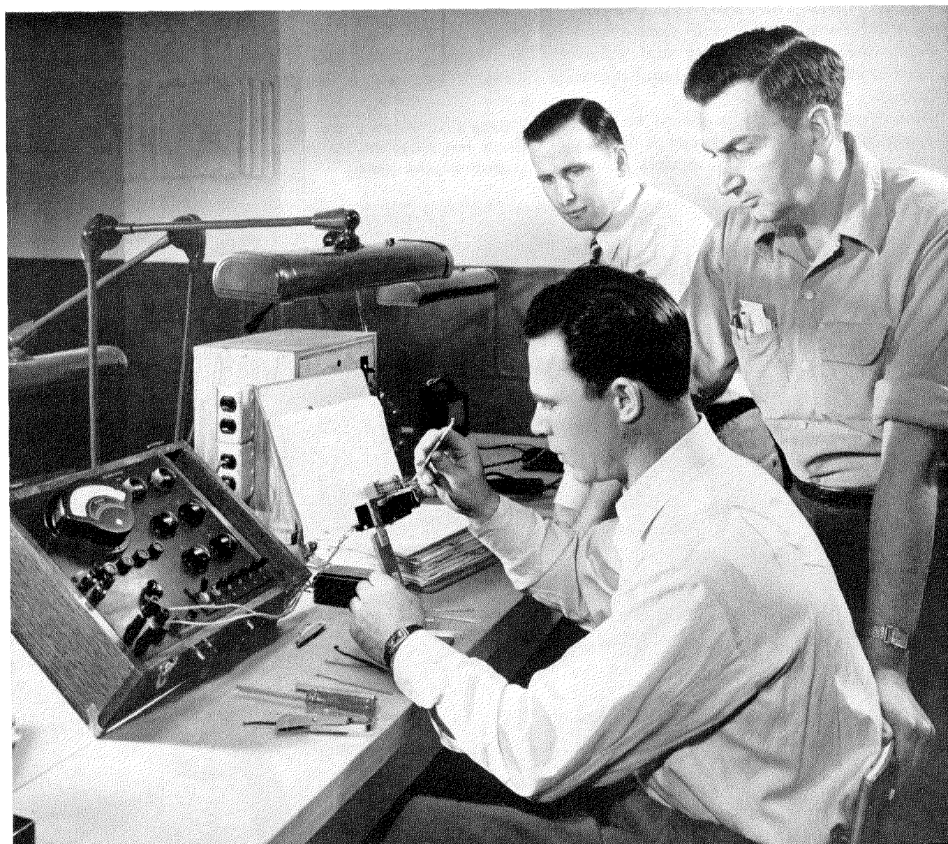
The type-4000 relay being adjusted here, the crossbar switch, and the magnetic impulse counter are crossbar dial-switching-system elements whose design is based on the simple movement of a relay armature. A Kellogg current-flow test set is being used in this operation.
