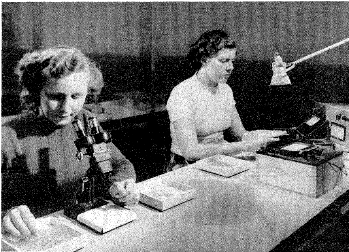
Figure 7—Above, sealing 1A thermistors into protective glass tubes.
