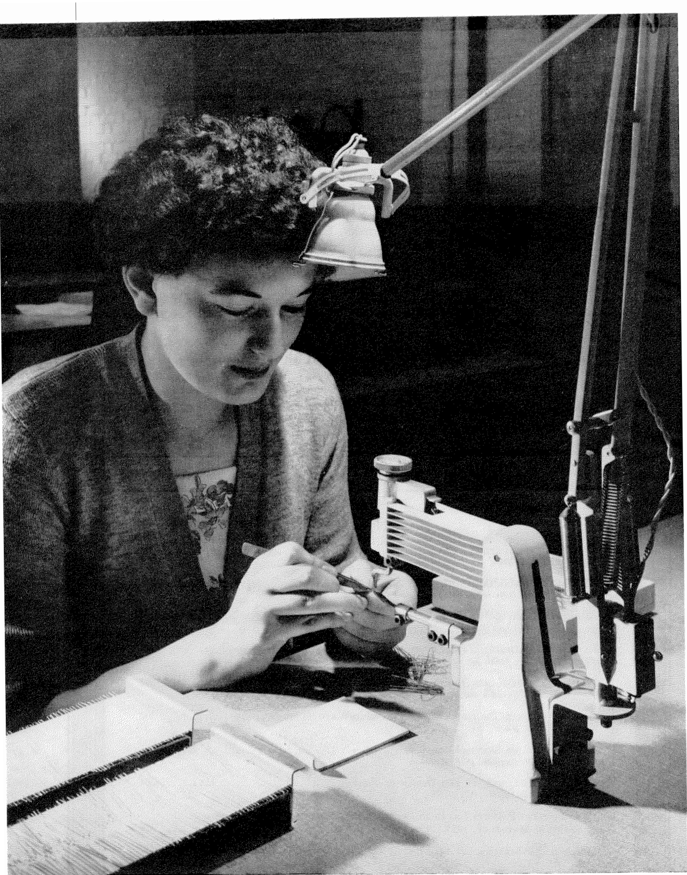
Welding the connecting wires to 1A thermistors.
