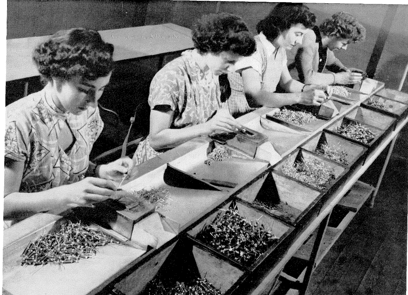
Figure 4—Soldering wires to Brimistors.
