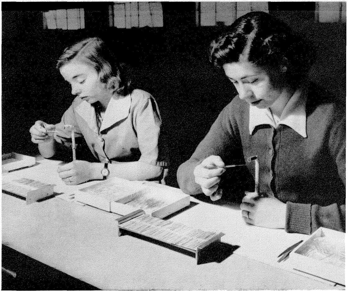
Figure 7—Above, sealing 1A thermistors into protective glass tubes.
