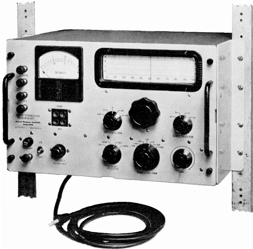
Figure 2—Rack mounting of set. The handles used for portable operation may be fastened into the cover, which is not used in this arrangement.
