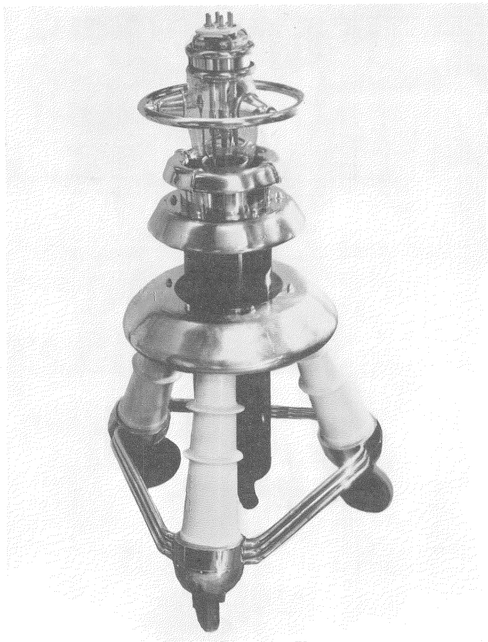
HUGE VACUUM TUBE DESIGNED BY I. T. & T. TWO TUBES ARE CAPABLE OF DELIVERING 200 KILOWATT CARRIER ON SHORTWAVE RADIO-TELEPHONY. THE HEIGHT OF THE TYPE WITH SUPPORTING "TRUCK," SHOWN IN THE ILLUSTRATION, IS FIVE FEET; THAT OF THE TUBE ITSELF IS FOUR FEET. PLANS FOR THE PRODUCTION OF THESE TUBES ARE BEING FORMULATED.
