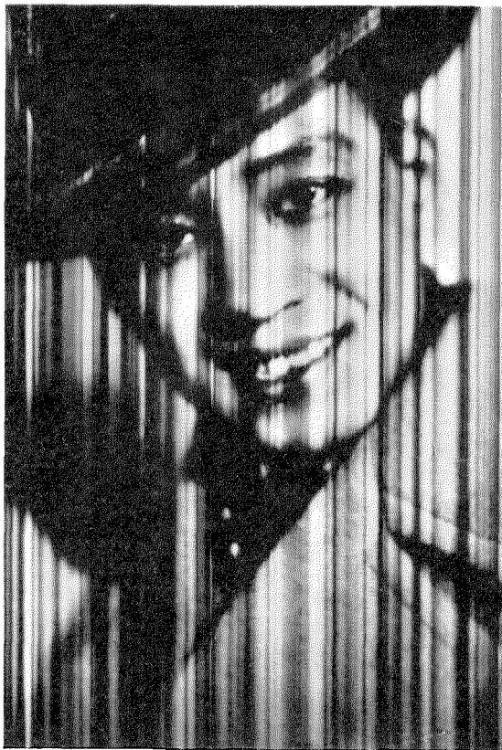
Fig. 1—Effect of Fading on Picture Transmitted Using Amplitude Modulation.
