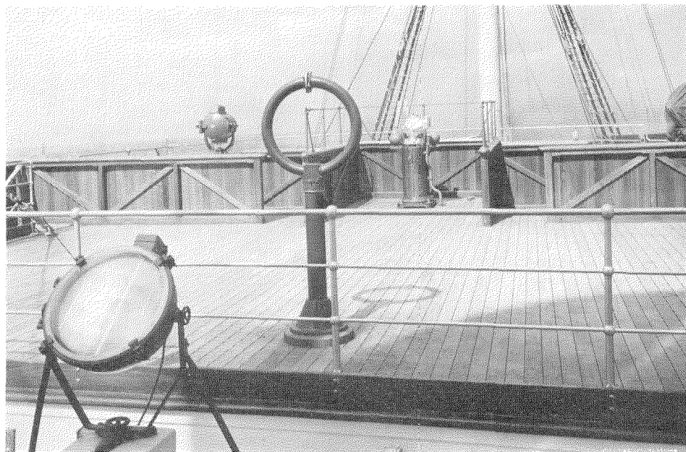
Rotating Loop Portion of the I.M.R.C. Radio Direction Finder Installed on the Bridge of the R.M.S. Queen Mary.
