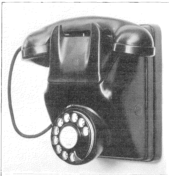
Fig. 4—Universal Telephone Set Arranged for Automatic Wall Mounting.
