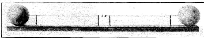
Figure 3—The First Oscillator of Hertz. Two copper wires, each 1 metre in length, supported on rods of sealing wax. The large spheres are of sheet zinc, and are 30 centimetres in diameter. Base 260 x 7.5 centimetres
