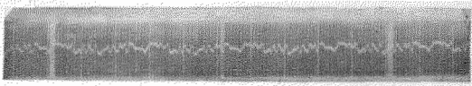
Figure 6—Test Message. Signals received April 16, 1920, over coil-loaded artificial line equivalent to a 1,700 n.m. cable with 30 m.h./n.m. Speed, 2,240 letters per minute
