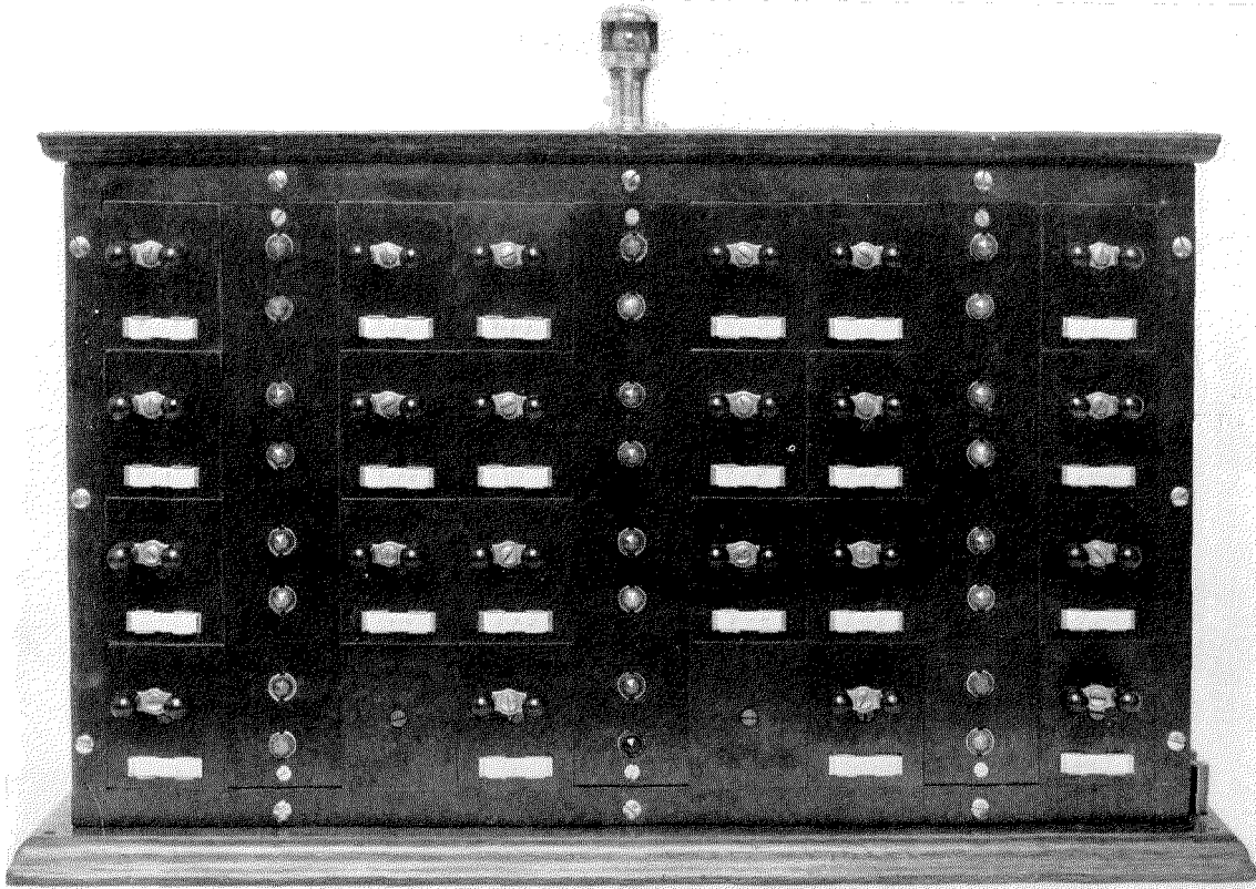
Figure 2E—Selector System, Dispatcher's Station Equipment—Key and Lamp Cabinet Located on Dispatcher's Desk. Contains Two Keys and Two Lamps for Each Unit Supervised. One of These Keys Will Open While the Other Will Close a Circuit Breaker. One Lamp (Green) Indicates the Open Position, the Other Lamp (Red) Indicates the Closed Position of the Unit Supervised
