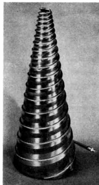
Fig. 8—Conical balanced equiangular spiral antenna.
