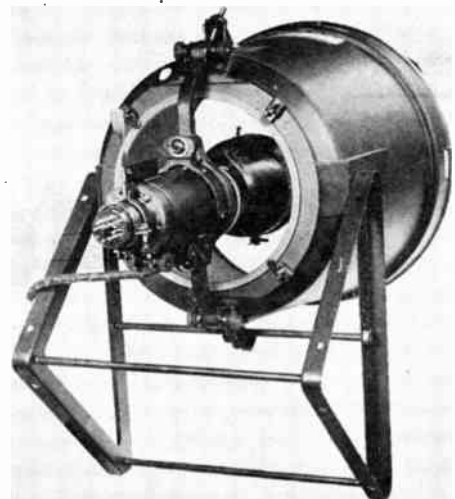
Fig. 13—Television-receiver designers achieved large picture sizes in various ways. The Philco projection receiver (circa 1948) gave the largest picture of any home receiver at the time, using Schmidt optics (shown here) to enlarge the picture from a 4-in diameter tube. Ingenious principles were used to gain picture size equivalent to that from a 24-in tube with equal brilliance at a nominal cost.
