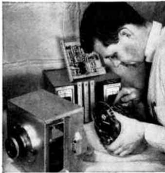
STAR-FIELD TRACKER correlates a viewed star pattern against a stored reference map for spacecraft attitude control. This device may replace the inertial table as an attitude sensor because of its zero drift.
