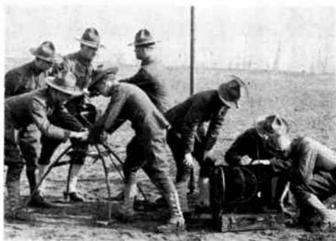
Fig. 7—Signal Corps field set developed during World War I. A spark set powered by hand-driven generator.
