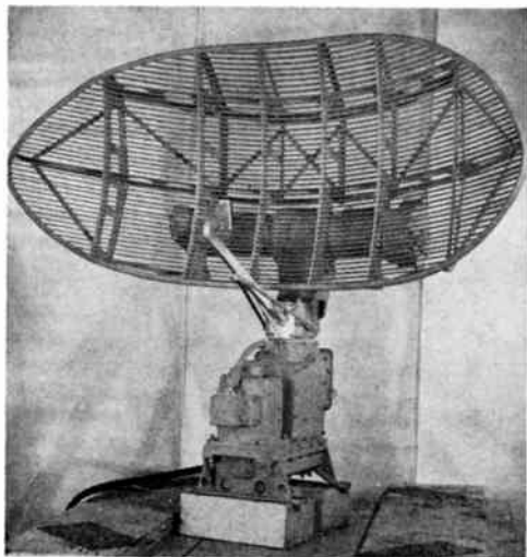
Fig. 2—Antenna with asymmetrically cut reflector.
