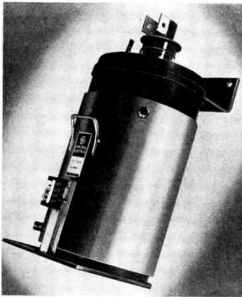
Fig. 6—Locomotive rectifier. Body length 23\frac{1}{4} inches; peak anode current = 2500 amperes; peak fault current = 40,000 amperes; maximum peak anode voltage = 4,000 volts.
