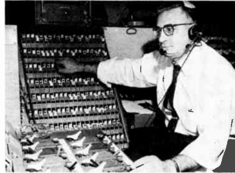
Fig. 5—Solid-state silicon controlled rectifier dimmers with punch-card preset control.
