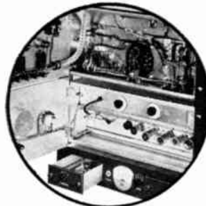
Individual drawer type modules for solid state modulator
