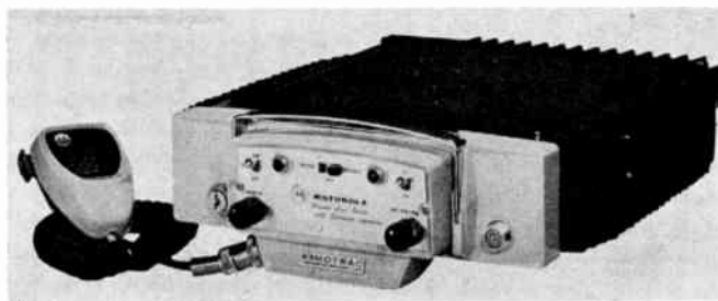
Fig. 5—The 1961 mobile FM station with transistorized receiver and power supply.
