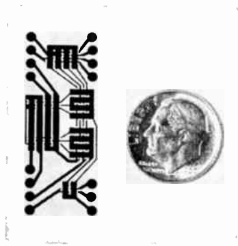
CRYOGENIC PROGRESS in inertial guidance is typified by this 32-gate logic element for smaller, faster, more reliable computers. Other current cryogenic work includes high-precision gyros and accelerometers.
