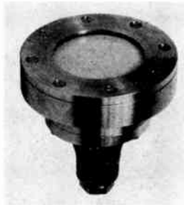
Fig. 8—Photograph of transducer for liquid level indicator (3° beam angle—negligible secondary lobes.)
