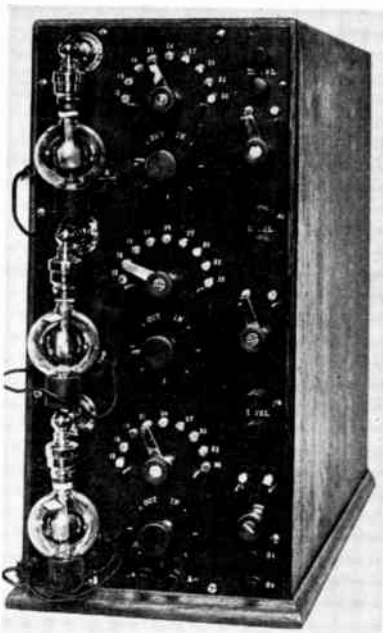
Fig. 2—Three-stage De Forest audion amplifier of the type first built in 1912 by the Federal Telegraph Company. This is the earliest known cascade AF amplifier. Tests made at that time indicated that the amplifier increased the received signal intensity by 120 times. (Courtesy of ITT.)
