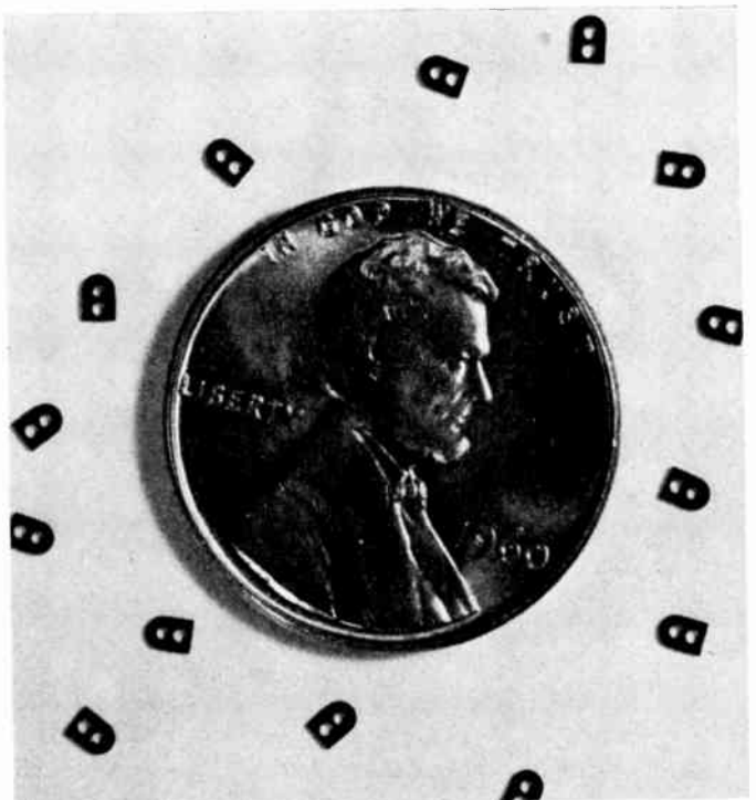
Fig. 11—Ferrite cores for random-access memory for NASA's Orbiting Astronomical Observatory (IBM).
