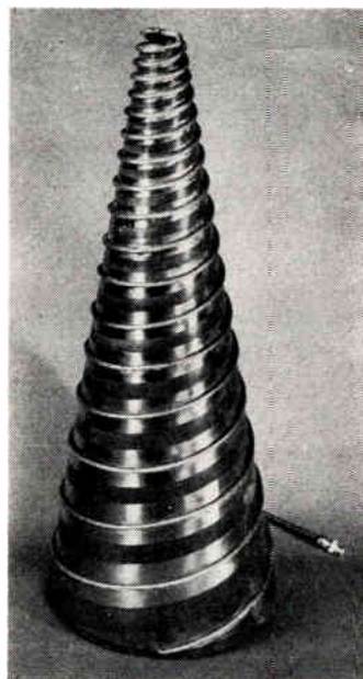
Fig. 8—Conical balanced equiangular spiral antenna.
