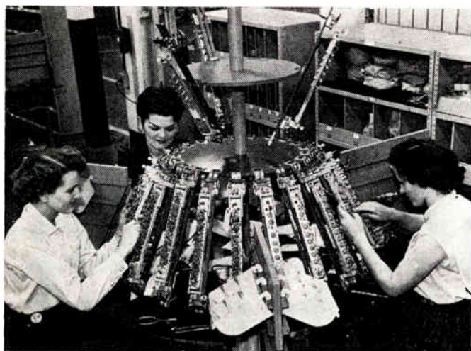
Fig. 17—"Wheel of fortune" lazy Susan assembly fixture, a methodizing approach first used successfully about 1955 to assemble Matador IF strips (and other similar assemblies) at The Martin plant in Baltimore, Md.
