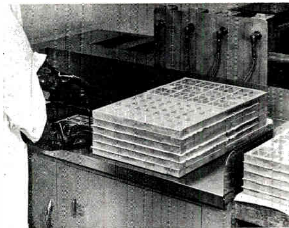
Fig. 10—Photograph of ultrasonic cleaning in production line.
