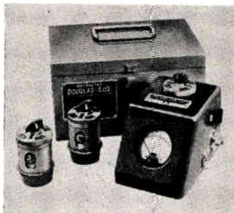
THE DOUGLAS MODEL 502, BI-DIRECTIONAL POWER MONITORS, are compact, versatile instruments, which are used for intermittent or continuous measuring of incident and reflected power or for precise, convenient matching of loads to lines. These instruments are designed to operate in a 50 ohm coaxial systems and normally are supplied with Type N connectors.
