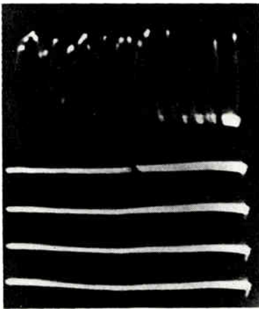
Fig. 6—Echoes of ground clutter (first line, 10 miles) and airplanes (second line, range about 15 miles) with 80-Mc radar installed with duplexer in field house. 5-Line sweep, 10 miles per line—total, 50-mile time base. December, 1936.
