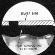
Enlarged section of Elastaclamp's inner cartridge.
